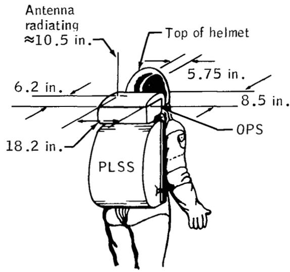
Figure 2. - Antenna mounting on the OPS.
