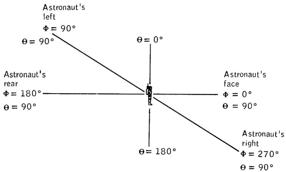
Figure 5. - Pattern coordinate system.
