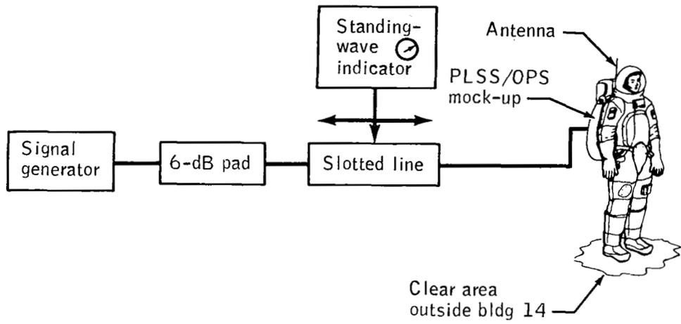
Figure 1. - The VSWR test setup.
