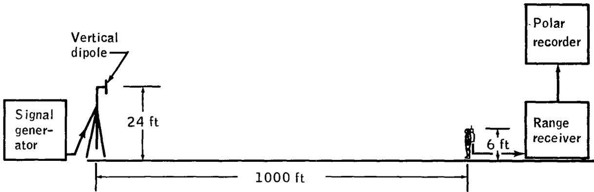
Figure 3. - Antenna pattern setup.
