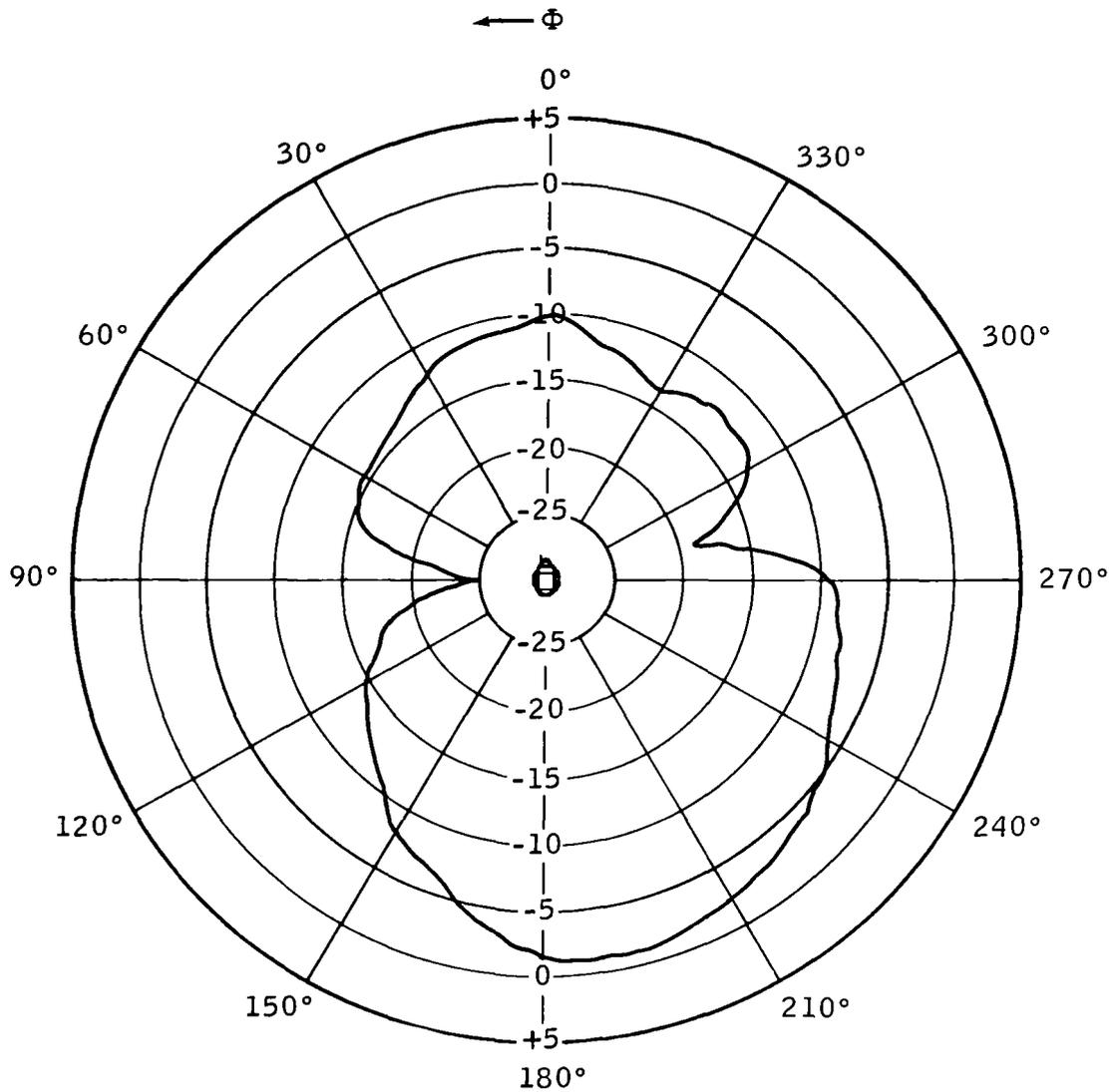
The gains are referenced to a perfect isotropic level of vertical-linear polarization established at the 6-foot standing height by substitution of a reference dipole.
