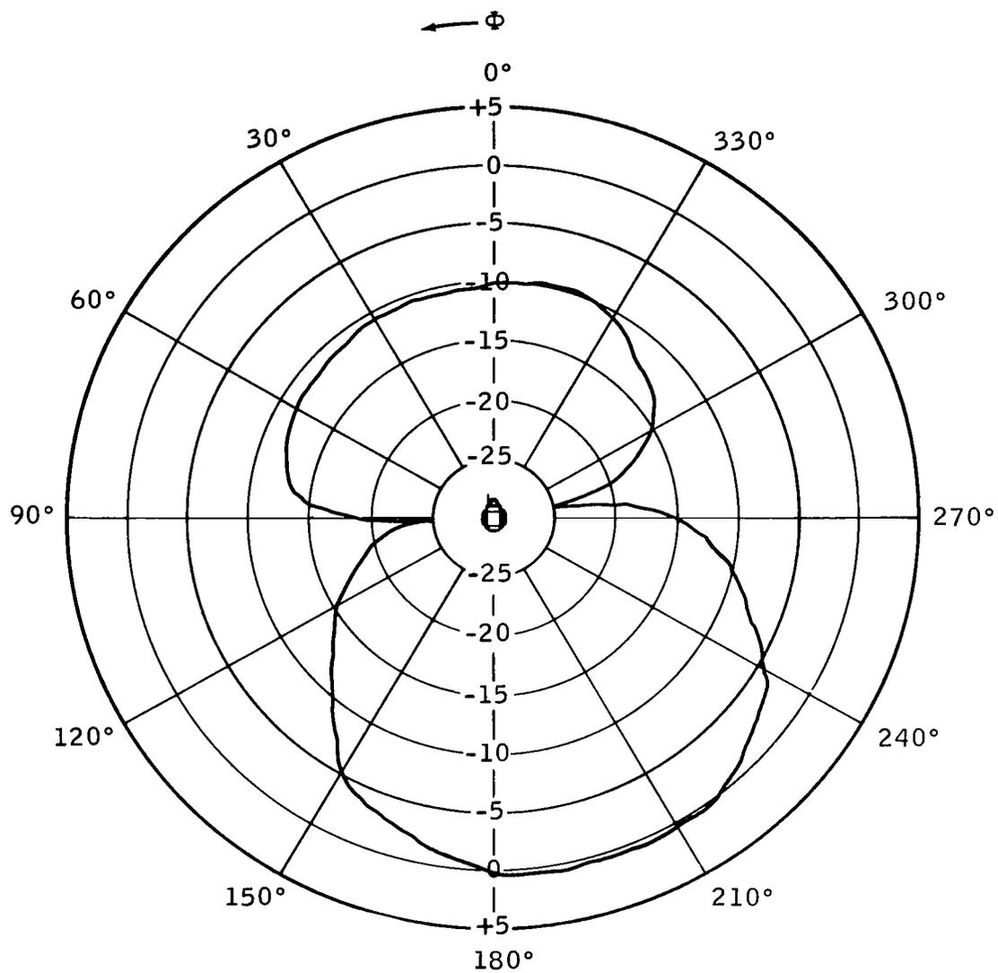
The gains are referenced to a perfect isotropic level of vertical-linear polarization established at the 6-foot standing height by substitution of a reference dipole.
