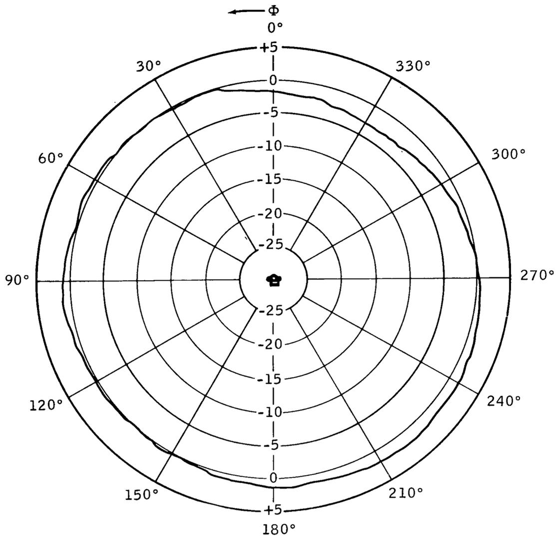
The gains are referenced to a perfect isotropic level of vertical-linear polarization established by substitution of a reference dipole for the backpack antenna.
