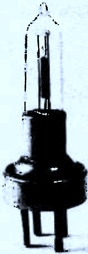
A Mullard "Weco" valve, produced around 1925. Its filament consumed 0.25 amp at 1 volt, and was normally powered by a single dry cell via a rheostat. The rheostat was adjusted to allow for voltage change as the battery ran down (courtesy Mullard Ltd.)
