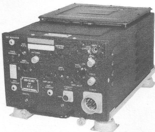
Figure 82. The r-f section of the first BLOCK III Transmitter used a push-pull master oscillator and power amplifier, but no buffer stage.
