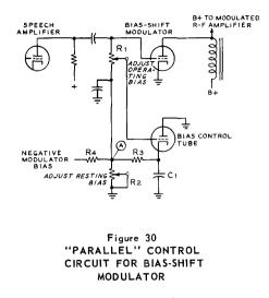
The resistance to ground of point A in the bias network is varied at a syllabic rate by the bias control tube.
