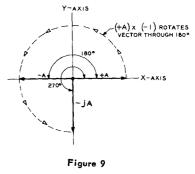
Operation on the vector (+A) by the quantity (-1) causes vector to rotate through 180 degrees.
