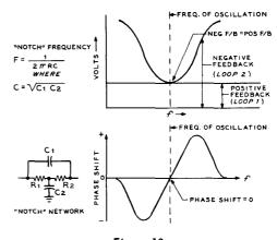
Figure 19 BRIDGE-T FEEDBACK LOOP CIRCUITS
