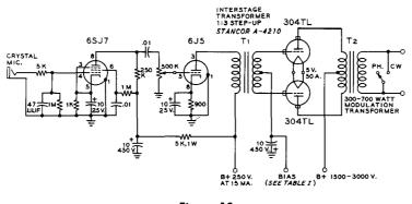
Figure 13 PUSH-PULL 304TL CLASS AB<sub>1</sub>, MODULATOR
