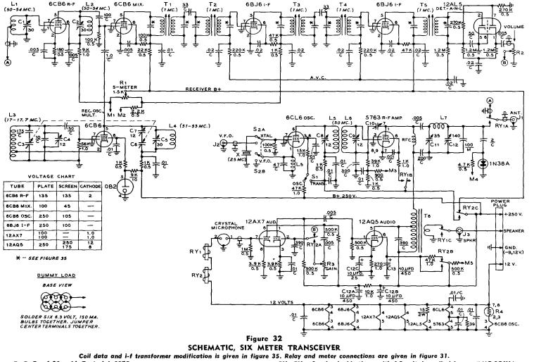
C1-C2-C5-6-30 µµfd. Centralab 827C C4-C7-S8-C9-3-12 µµfd. Centralab 827B C<sub>3</sub>-C<sub>6</sub>-15  $\mu\mu$ fd. per section. All-Star Products Co., Defiance, Ohio. Model C3 -7 µµfd. variable "piston-type". Erie 532B C 10 25 ....td Hammarlund HF-35
