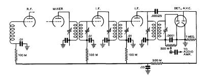
Figure 26 TYPICAL A-V-C CIRCUIT USING A DOUBLE DIODE Any of the small dual-diode tubes may be used in this circuit. Or, if desired, a duo-diodetriode may be used, with the triode acting as the first audio stage. The left-hand diode serves as the detector, while the right-hand side acts as the a-v-c rectifier. The use of separate diodes for detector and a-v-c reduces distortion when receiving an AM signal with a high
