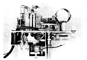
occupies the far end of the chassis. Pi-network switch  $S_2$  is placed next to the tuning capacitor, and the various padding capacitors are mounted directly on the back of the switch section.
