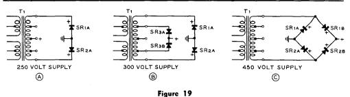
SIMPLIFIED CIRCUITS OF RECTIFIER SYSTEMS USED IN HIGH EFFICIENCY MOBILE SUPPLY
