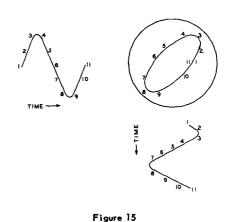
PROJECTION DRAWING SHOWING THE RE-SULTANT PHASE DIFFERENCE PATTERN OF TWO SINE WAVES 45° OUT OF PHASE
