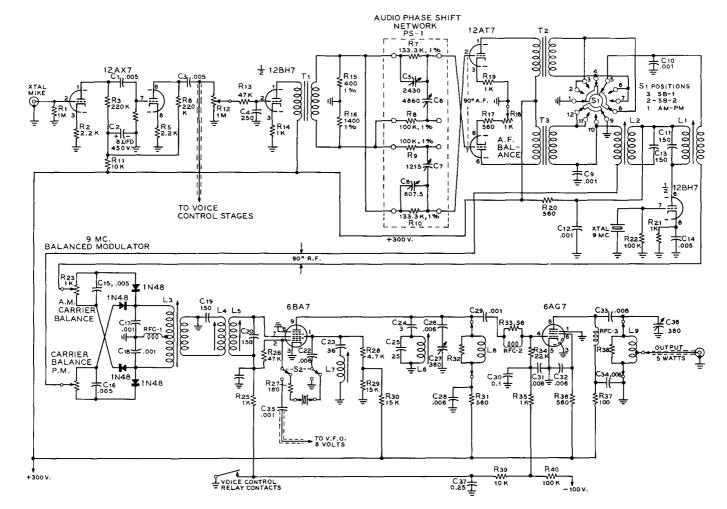
Figure 37 SIMPLIFIED SCHEMATIC OF "TEN-A" EXCITER 348 Sideband Transmission
