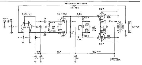
Figure 19 U. S. VERSION OF BRITISH "WILLIAMSON" AMPLIFIER PROVIDES 10 WATTS POWER OUTPUT AT LESS THAN 2% INTERMODULATION DISTORTION. 6SN7 STAGE USES DIRECT COUPLING.
