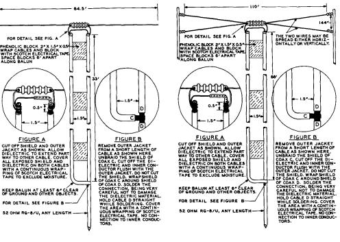
DIMENSIONS SHOWN HERE ARE FOR THE 40 METER BAND. THIS ANT-ENNA MAY BE BUILT FOR OTHER BANDS BY USING DIMENSIONS THAT ARE MULTIPLES OR SUBMULTIPLES OF THE DIMENSIONS SHOWN. BALUN SPACING IS 1.5° ON ALL BANDS.
