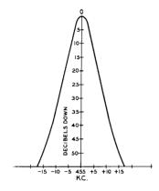
Figure 15 I-F PASS BAND OF TYPICAL COMMUNICATIONS RECEIVER
