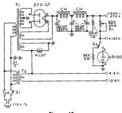
Figure 42 SCHEMATIC, LIGHT DUTY SUPPLY 7.—350-0-350 volts at 50 milliamperes, 5 volts at 2 amperes, 6.3 volts at 3 amperes, "replacement" transformer. 7.—6.3 volts at 1.2 amp. Stancor P-6134 CH—4.5 henry at 50 ma. Stancor C-1706
