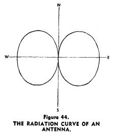
Polar coordinates are used principally in radio work for plotting the directional characteristics of an antenna where the radiation is represented by the distance of the curve from the origin for every possible direction.
