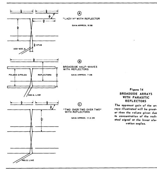
If six or more elements are used in the type of array shown in figure 15B no matching section will be required between the antenna transmission line and the feed point of the antenna. When only four elements are used the antenna is the familiar "lazy H" and a quarter-wave stub should be used for feeding from the antenna transmission line to the feed point of the antenna system.
