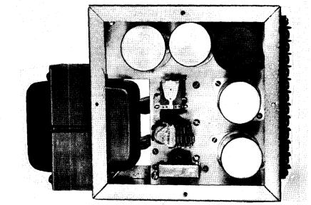
Figure 22 TOP VIEW OF POWER SUPPLY INTERIOR
