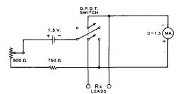
Figure 3 SCHEMATIC OF A LOW-RANGE OHMMETER
