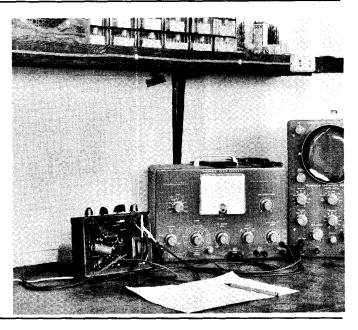
Figure 25 TYPICAL INTERMODULATION TEST OF AUDIO AMPLIFIER. Audio tones of two frequencies are applied to input of amplifier under test, and amplitude of "sum" or "difference" frequency is measured, providing relative inter-modulation figure.
