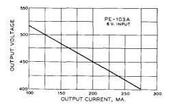
Figure 11 APPROXIMATE OUTPUT VOLTAGE VS. LOAD CURRENT FOR A PE-103A DYNAMOTOR
