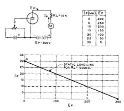
Figure 11 The static load line for a typical triode tube with a plate load resistance of 10,000 ohms.
