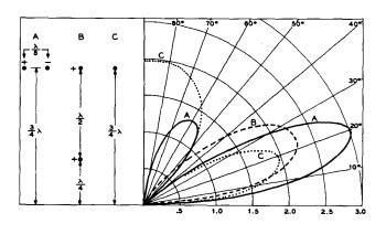
angle radiation at the expense of the useless high-angle radiation with these simple arrays as contrasted to the dipole is quite marked.
