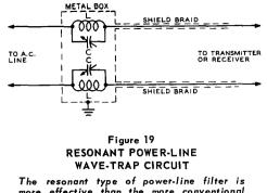
more effective than the more conventional "brute force" type of line filter, but requires tuning to the operating frequency of the transmitter.
