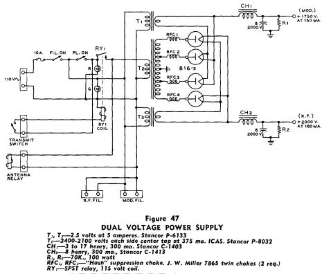
. RFC:------Hash" suppression choke. J. W. Miller 7865 twin chokes (2 req.) -SPST relay, 115 volt coil.
