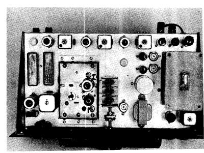
age regulator tube, and the 12AU7 S-meter tube. In front of the last i-f transformer can are the two 6AL5 tubes and potentiometers  $R_s$  and  $R_{s}$ .
