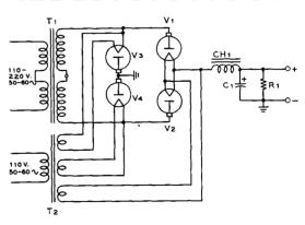
Figure 40 HIGH-VOLTAGE POWER SUPPLY
