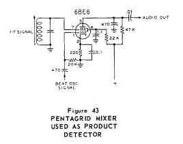
Such a detector is useful for single sideband work, since the inter-modulation distortion is extremely low.
