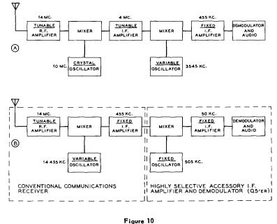
TYPICAL DOUBLE-CONVERSION SUPERHETERODYNE RECEIVERS Illustrated at (A) is the basic circuit of a commercial double-conversion superheterodyne receiver. At (B) is illustrated the application of an accessory sharp i-f channel for obtaining improved selectivity from a conventional communications receiver through the use of the double-conversion principle.
