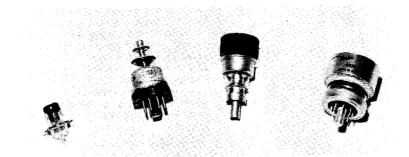
Figure 2 V-H-F and U-H-F TUBE TYPES
