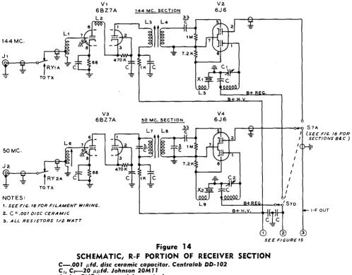
C\_\_OG\_\_μ(J), usic cervine copients. Contrained Dis-Tox J,, J\_\_\_BNC-type coaxial receptacle L<sub>1</sub>-L<sub>2</sub>-\_See figure 21 for coil information S7A, D\_\_Part of S7 (Centralab wafer PA-9) See figure 18. RY<sub>1</sub>A, RY<sub>2</sub>A-See figure 19 X<sub>1</sub>--114 Mc. overtone crystal. Precision Crystal Lab., Santa Monica, Calif. X<sub>2</sub>--84 Mc. crystal (see X<sub>1</sub>)
