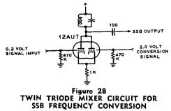
push-pull circuits and the tubes into exact amplitude and phase balance, about 20 db of injection frequency cancellation is all that can be depended upon. With suitable trimming adjustments the cancellation can be made as high as 40 db, however, in fixed frequency circuits.
