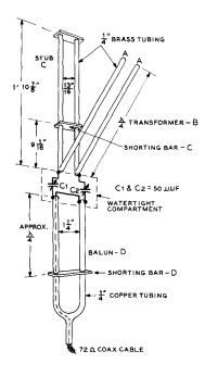
Figure 17 THE MATCHING UNIT IN DETAIL FOR THE PE1PL BEAM DESIGN, WHICH AL-LOWS THE USE OF 72-OHM COAX
