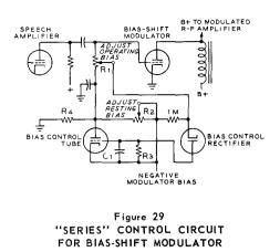
The internal resistance of the bias control tube is varied at a syllabic rate to change the operating bias of the modulator tube.
