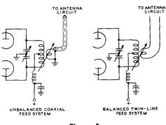
Figure 1 LINK COUPLED OUTPUT CIRCUITS FOR PUSH-PULL AMPLIFIERS
