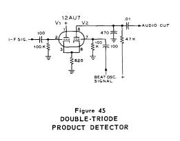
"plate" detector, the cathode of which is common with the cathode follower amplifier. The local oscillator signal is injected into the grid circuit of tube V2.
