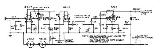
Figure 9 FM REACTANCE MODULATOR WITH SPEECH CLIPPER
