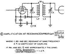
MAXIMUM AMPLITUDE OCCURS AT CRITICAL COUPLING -WHEN K =  $\sqrt{\frac{1}{\sqrt{QP}Qs}}$
