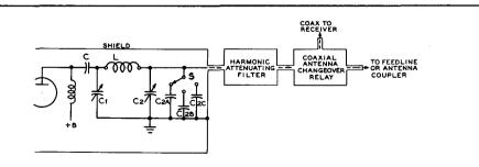
Figure 38 PI-NETWORK ANTENNA COUPLER
