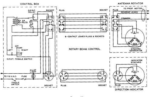
Figure 21 SCHEMATIC OF A COMPLETE ANTENNA CONTROL SYSTEM
