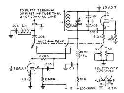
L1= GRAYBURNE V6 CHOKE (0.6-6.0 MH) L2= GRAYBURNE "LOOPSTICK" COIL
