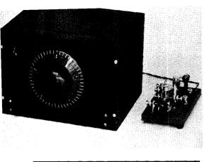
up wih a dummy load. This will provide injecton signal for proper receiver operation at 220.1 Mc. A remote signal (preferably that of the companion unit) should be used as a signal source and the tuned circuits of the r-f amplifiers adjusted for best signal reception. It may be necessary to alter the spacing of coils L<sub>8</sub>-L<sub>11</sub> to provide proper circuit resonance which should occur at about the middle of the tuning range of the associated capacitor.
