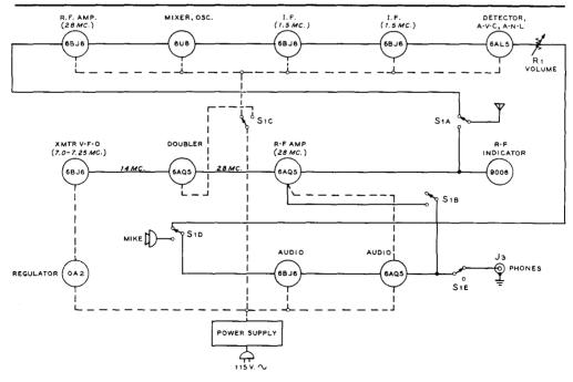
Figure 37 BLOCK DIAGRAM OF TEN METER TRANSCEIVER
