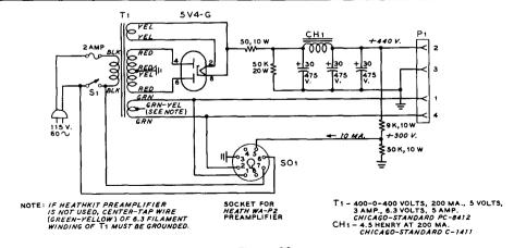
Figure 30 POWER SUPPLY FOR 20-WATT AMPLIFIER.
