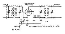
Figure 6 TYPICAL I-F AMPLIFIER STAGE
