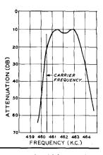
characteristics of the mechanical filter. For simplicity, the mixing and filtering operation usually takes place at a frequency of 455 kilocycles. The single-sideband signal appearing at the output of the mechanical filter may be translated directly to a higher operating frequency. Suitable tuned circuits must follow the conversion stage to eliminate the signal from the conversion oscillator.
