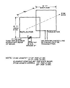
Figure 20 THE CUBICAL-QUAD ANTENNA FOR THE 10-METER BAND
