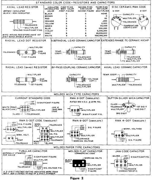
STANDARD COLOR CODE FOR RESISTORS AND CAPACITORS
