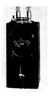
Figure 25 SIMPLE SILICON CRYSTAL NOISE GENERATOR
