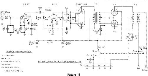
SCHEMATIC OF BEAM POWER TUBE MODULATOR M-0 - 250 d.c. milliammeter Tr
