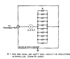
Figure 8 1.6-KILOWATT DUMMY LOAD SCHEMATIC
