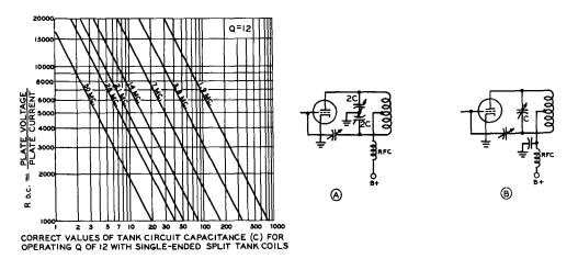
Figure 24 PLATE-TANK CIRCUIT ARRANGEMENTS
