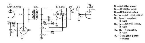
Figure 30 NOISE LIMITER CIRCUIT, WITH ASSOCIATED A-V-C This limiter is of the series type, and is self-adjusting to carrier strength for phone reception. For proper operation several volts should be developed across the secondary of the last i-f transformer (IFT) under carrier conditions.
