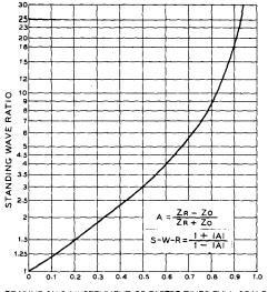
READING ON 0-1 INSTRUMENT, OR FACTOR TIMES FULL SCALE (MAGNITUDE OF REFLECTION COEFFICIENT, A)
