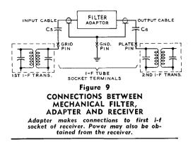
tuted for the first 455 kc. intermediate frequency amplifier tube, without making any under-chassis changes in the receiver. Simply connect the adapter to a power source (which may be your receiver), remove the first i-f amplifier tube, and insert two short coaxial cables into the empty tube socket, as shown in figure 9. These cables carry the i-f signal to and from the adapter, which are then tucked away in an unoccupied corner of your receiver or speaker cabinet.
