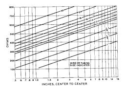
Figure 20 CHARACTERISTIC IMPEDANCE OF TYPI-CAL TWO-WIRE OPEN LINES
