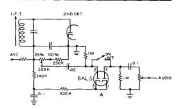
Figure 32 THE FULL-WAVE SERIES AUDIO NOISE LIMITER
