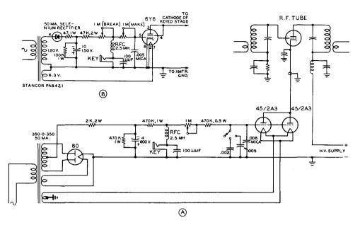
Figure 10 VACUUM TUBE KEYERS FOR CENTER-TAP KEYING CIRCUITS
