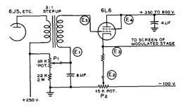
Figure 5 CATHODE-FOLLOWER SCREEN-MODULATION CIRCUIT
