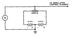
Figure 10 REACTANCE-TUBE LINEARITY CHECKER
