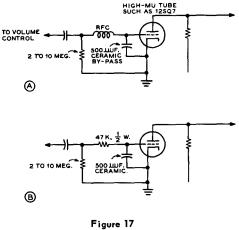
CIRCUITS FOR ELIMINATING AUDIO-STAGE RECTIFICATION
