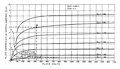
Figure 7 AVERAGE PLATE CHARACTERISTICS OF 813 TUBE
