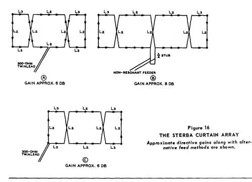
sent points of maximum current. All arrows should point in the same direction in each portion of the radiating sections of an antenna in order to provide a field in phase for broadside radiation. This condition is satisfied for the arrays illustrated in figure 16. Figures 16A and 16C show simple methods of feeding a short Sterba curtain, while an alternative method of feed is shown in the higher gain antenna of figure 16B.
