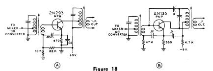
TRANSISTORIZED I-F AMPLIFIERS. Typical P-N-P transistor must be neutralized because of high collector capacitance. Rate grown N-P-N transistor does not usually require external neutralizing circuit.
