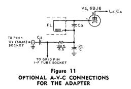
overloading when no plate current flows through the input coil. Both filter coils are tuned to resonance at the intermediate frequency by fixed capacitors  $C_2$  and  $C_3$ .
