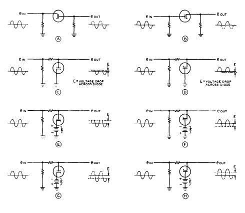
Figure 1 VARIOUS DIODE LIMITING CIRCUITS
