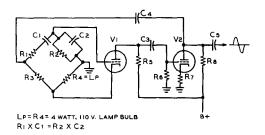
Figure 15 THE WIEN-BRIDGE AUDIO OSCILLATOR
