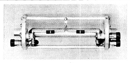
Figure 16 INTERIOR VIEW OF COAXIAL REFLECTOMETER
