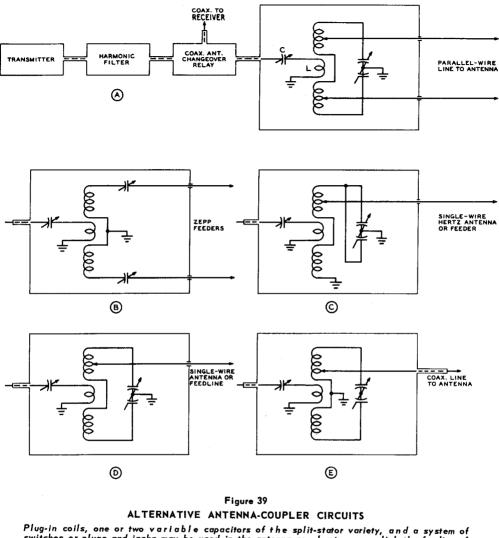
switches or plugs and jacks may be used in the antenna coupler to accomplish the feeding of different types of antennas and antenna transmission lines from the coaxial input line from the transmitter or from the antenna changeover relay. Link L should be resonated with capacitor C at the operating frequency of the transmitter so that the harmonic filter will operate into a resistive load impedance of the correct nominal value.
