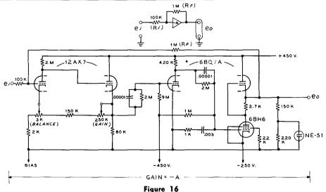
HIGH GAIN OPERATIONAL AMPLIFIER, SUCH AS USED IN HEATH COMPUTER.
