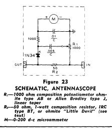
nected across the bridge, it will indicate a voltage null at bridge balance. The radiation resistance of the antenna may then be read directly from the calibrated resistor of the instrument.
