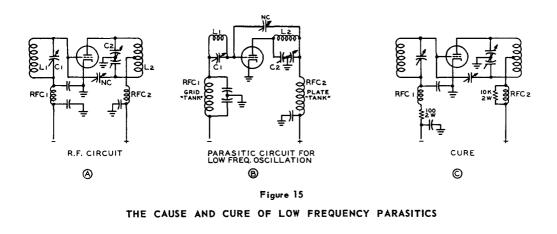
of such tubes. Try larger and smaller screen by-pass capacitors to determine whether or not they have any effect. If the condition is coming from the screen circuit an audio choke with a resistor across it in series with the screen feed lead will often eliminate the trouble.
