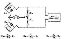
$$\label{eq:standard} \begin{split} Z_X &= \mathsf{IMPEDANCE} \text{ Being measured, } R_S = \mathsf{resistance component of } Z_S\\ Z_S &= \mathsf{IMPEDANCE OF STANDARD, } X_X = \mathsf{reactance component of } Z_X\\ R_X &= \mathsf{Resistance component of } Z_X, X_S = \mathsf{reactance component of } Z_S \\ \end{split}$$
