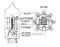
Figure 4 CUT-AWAY DRAWING OF A 6CB6 PENTODE
