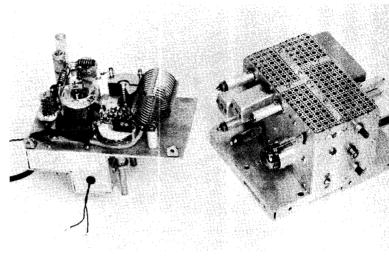
clearly visible in figure 32. The clearance space provided by the "step" is occupied by the "SSB- standby-CW" switch S1 which is mounted to the panel in close proximity to the grid circuit components of the amplifier stage. The important leads to the control switch pass out of the grid compartment through ceramic feed through capacitors mounted on the wall of the "step" shield. The coaxial r-f output lead and the grid bias lead also pass through this shield and may be seen in figure 32.
