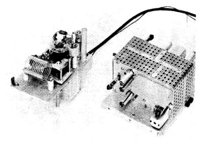
ployed with the linear amplifier stage. In order to conserve space, the usual variable capacitor is omitted from the output side of the network and a rotary switch and selection of fixed capacitors is employed in its place. Proper choice of capacitors permits the transmitter to be matched to 52- or 72-ohm transmission lines having s.w.r. values as great as 2.5/1.
