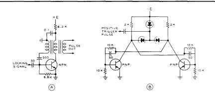
Figure 26 TRANSISTORIZED BLOCKING OSCILLATOR (A) AND ECCLES-JORDAN BI-STABLE MULTIVIBRATOR (B). High-alpha transistors must be employed in counting circuits to reduce effects of storage time caused by transit lag in transistor base.
