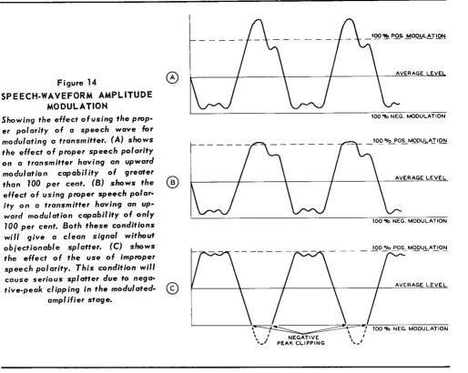
negative peaks of modulation. This aspect of the problem has been discussed in more detail in the section on *Speech Waveform Dissymmetry* earlier in this chapter. The effect of feeding the proper speech polarity from the speech amplifier is shown in figure 14.
