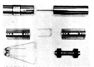
Figure 46 EXPLODED VIEW OF COLLINS MECHANICAL FILTER
