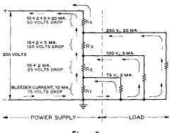
Figure 9 MORE COMPLEX VOLTAGE DIVIDER The method for computing the values of the resistors is discussed in the accompanying text.
