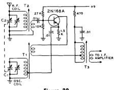
Figure 20 THE AUTODYNE CONVERTER CIRCUIT USING A 2N168A AS A MIXER.
