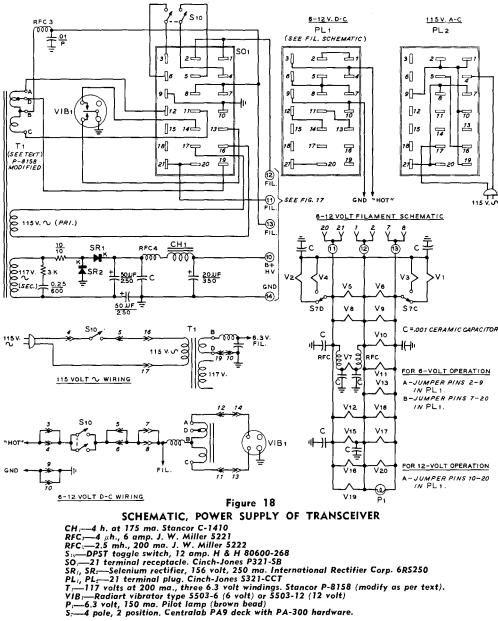
The power transformer is made from a TVreplacement type, with a new vibrator winding replacing the usual 6.3 volt filament windings. Information covering the conversion of the transformer will be found later in this section. The special winding may be arranged for either 6-volt d.c. or 12- volt d.c. operation, but not both. Thus, the choice of d.c. supply voltage must be determined before the transformer is modified.
