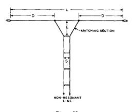
Figure 28 THE DELTA-MATCHED DIPOLE ANTENNA
