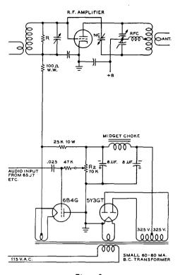
Figure 3 GRID-BIAS MODULATOR CIRCUIT
