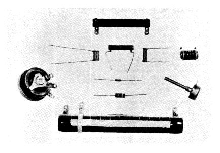
Figure 2 TYPICAL RESISTORS Shown above are various types of resistors used in electronic circuits. The larger units are power resistors. On the left is a variable power resistor. Three precision-type resistors are shown in the center with two small composition resistors beneath them. At the right is a composition-type potentiometer, used for audio circuity.
