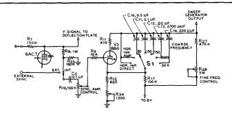
Figure 5 SCHEMATIC OF SWEEP GENERATOR
