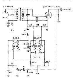
Figure 33 THE TNS AUDIO NOISE LIMITER
