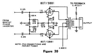
"ULTRA-LINEAR" CONFIGURATION OF WILLIAMSON AMPLIFIER DOUBLES POWER OUT-PUT, AND REDUCES IM LEVEL. SCREEN TAPS ON OUTPUT TRANSFORMER PERMIT "SEMI-TETRODE" OPERATION.
