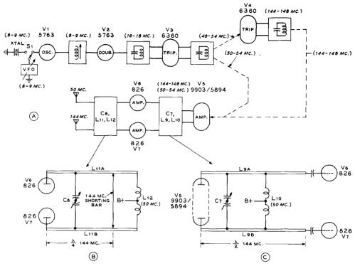
Figure 2 BLOCK DIAGRAM OF VHF TRANSMITTER
