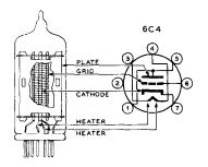
Figure 3 CUT-AWAY DRAWING OF A 6C4 TRIODE
