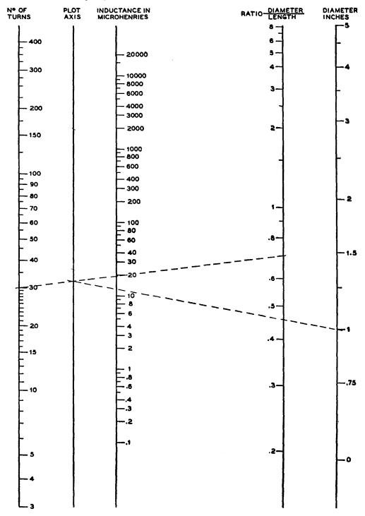
ductance, the D/L ratio, and the diameter are known, simply work backwards from the example given. In all cases, remember that the straightedge reads either turns and D/L ratio, or it reads inductance and diameter. It can read no other combination.
