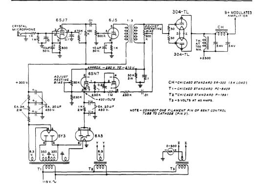
Figure 31 500-WATT BIAS SHIFT MODULATOR
