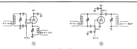
Figure 1 SIMILAR CATHODE FOLLOWER CIRCUITS HAVING DIFFERENT R-F GROUND POINTS.
