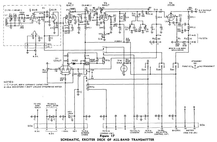
C<sub>1</sub>-300  $\mu\mu$ fd. Bud CE-2008 dual bearing capacitor
