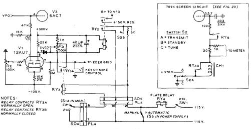
Figure 21 KEYER AND CONTROL CIRCUITS Clickless, break-in keying is provided by this simple control circuit. See text for full details of operation
