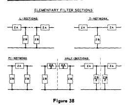
Complex filters may be made up from these basic filter sections.
