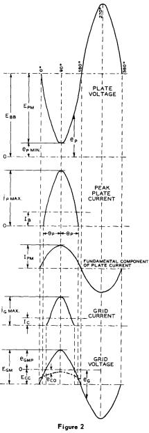
Instantaneous electrode and tank circuit voltages and currents for a Class C r-f power amplifier
