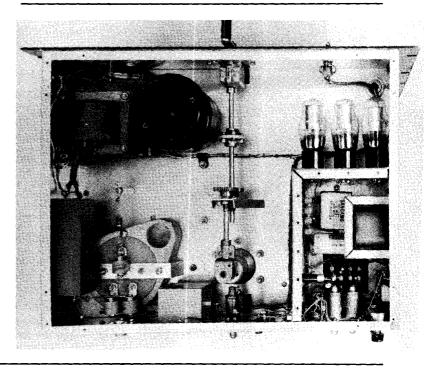
shield is 95%" high. This shield is made of one piece of aluminum, bent into a U-shape, having  $\frac{1}{2}$ -inch flanges on all sides. The open side of the "U" is bolted to the front panel as shown in the photographs. Elastic stop-nuts are affixed to the shield every  $1\frac{1}{2}$ " along the flange, or it may be drilled and tapped for 6-32 machine screws. A shield of this type can be homemade, or it may be fabricated in any large sheet metal shop for a small sum.
