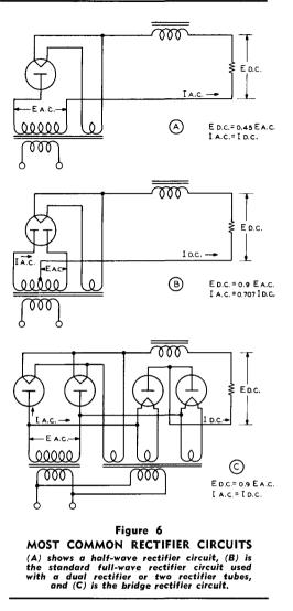
half of the rectified a-c wave is combined in the output as shown in figure 7. This pulsating unidirectional current can be filtered to any desired degree, depending upon the particular application for which the power supply is designed.
