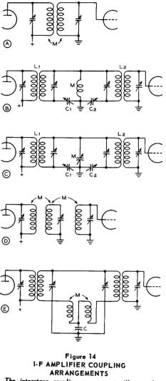
The interstage coupling arrangements illustrated above give a better shape factor (more straight sided selectivity curve) than would the same number of tuned circuits coupled by means of tubes.
