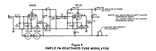
mounted in close proximity to the v.f.o. so that the lead from the 6CL6 to the grid circuit of the oscillator can be as short as possible. A practical solution is to mount the reactance modulator in a small box on the side of the v-f-o cabinet.
