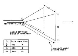
Figure 9 THE 60<sup>0</sup> HORN ANTENNA FOR USE ON FREQUENCIES ABOVE 144 MC.
