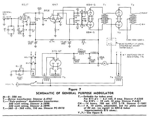
of the 500 watt modulator (figures 9 and 10) the size and weight of the components require that the speech amplifier be mounted on a separate chassis. For power levels of 300 watts or less it is possible to mount the complete speech system on one chassis.
