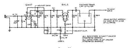
Figure 20 CLIPPER FILTER USING 6AL5 STAGE
