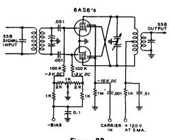
Figure 29 BALANCED MODULATOR CIRCUIT FOR SSB FREQUENCY CONVERSION
