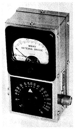
Figure 22 THE ANTENNASCOPE The radiation resistance of r-f loads connected across the output receptacle may be quickly determined by a direct dial reading. The Antennascope may be driven with a grid-dip oscillator, covering r-f impedance range of 5 to 1000 ohms.
