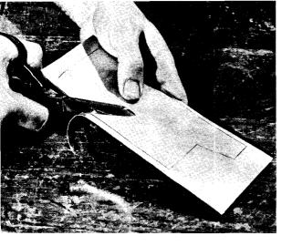
Figure 1 SOFT ALUMINUM SHEET MAY BE CUT WITH HEAVY KITCHEN SHEARS
