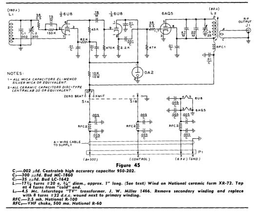
isolated both electrically and physically from the rest of the transmitting equipment. This goal cannot be achieved in practice since a vacuum tube or transistor must be coupled to these circuit elements to maintain oscillation. The coupling of such items deteriorates the electrical isolation of the frequency determining circuit. By the use of proper coupling circuits the effects of the tube or transistor can be minimized.
