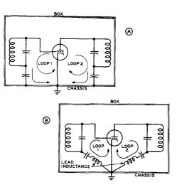
Figure 10 GROUND LOOPS IN AMPLIFIER STAGES
