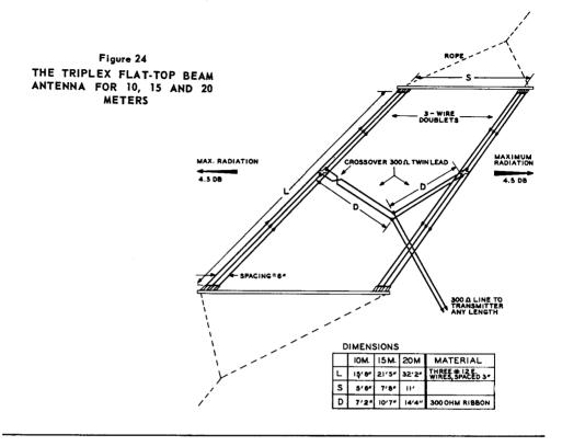
to one-quarter wave spacing may be used on the fundamental for the one-section types and also the two-section center-fed, but it is not desirable to use more than 0.15 wavelength spacing for the other types.
