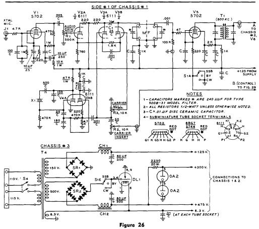
SCHEMATIC, LOW FREQUENCY SECTION AND POWER SUPPLY OF SSB TRANSMITTER DL .-
