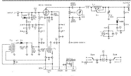
Figure 43 SCHEMATIC, 4CX-1000A LINEAR AMPLIFIER  $C_1$ —500 µµfd., 10KV variable vacuum capacitor. Jennings UCSL 4-500  $C_2$ —1500 µµfd., Cardwell 8013  $L_2$ -S<sub>1</sub>—High-C, all-band turret. Barker & Williamson 852 RFC<sub>1</sub>—2.5 mh. National R-100
