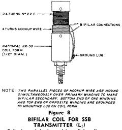
Coils L<sub>2</sub> and L<sub>3</sub> have 4-turn link coils over bottom end instead of the bifilar winding.
