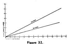
Only two points are needed to define functions which result in a straight line as shown in this diagram representing Ohm's Law.
