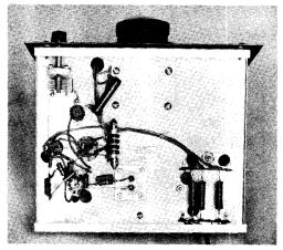
Figure 47 UNDER-CHASSIS VIEW OF V.F.O. UNIT
