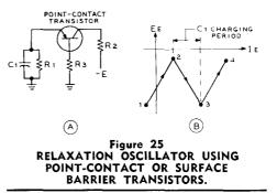
Relaxation Oscillators Transistors have almost unlimited use in relaxation and R-C oscillator service. The negative re-
