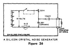
A simple means of determining the degree of actual sensitivity of a receiver is to inject a minute signal in the input circuit and then measure the amount of this signal that is needed to overcome the inherent receiver noise. The less injected signal needed to override the receiver noise by a certain, fixed amount, the more sensitive is the receiver.
