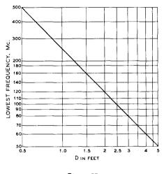
Figure 5B DESIGN CHART FOR THE "DISCONE" ANTENNA
