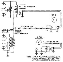
Figure 21 MONITORING CIRCUIT FOR TRAPEZOI-DAL MODULATION PATTERN
