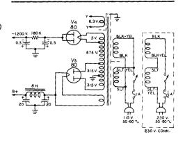
Figure 7 SCHEMATIC OF POWER SUPPLY
