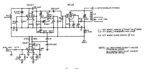
Figure 12 REACTANCE MODULATOR FOR 10, 15 AND 20 METER OPERATION
