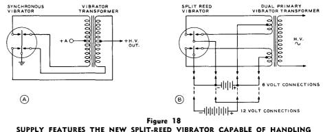
SUPPLY FEATURES THE NEW SPLIT-REED VIBRATOR CAPABLE OF HANDLING 100 WATTS OF POWER AT EITHER 6 OR 12 VOLTS
