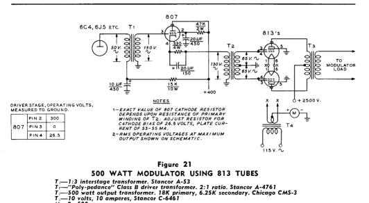
350 watts of audio are obtainable from this circuit at plate potential of 2000 volts.
