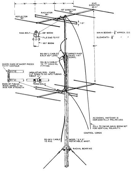
Figure 13 CONSTRUCTIONAL DRAWING OF AN EIGHT-ELEMENT TIPPABLE 144-MC. ARRAY
