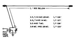
Figure 17 RECOMMENDED LENGTHS FOR THE END-FED HERTZ
