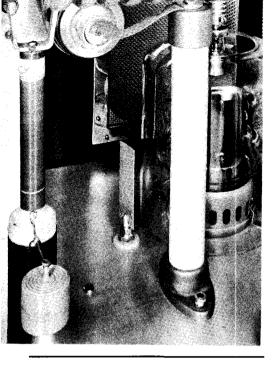
ets. It is necessary to ground the metal base ring of each tube to the chassis, since this ring forms part of the screen shielding circuit. If grounding clips are not furnished with the tube socket, they may be made from a short length of  $\frac{3}{8}$ -inch wide brass strap formed to spring against the base ring.
