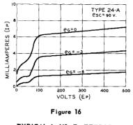
TYPICAL I<sub>p</sub> VS. E<sub>p</sub> TETRODE CHARACTERISTIC CURVES
