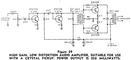
power may be obtained with a battery supply of 12 volts. Peak current drain under maximum signal conditions is 40 ma. Other interesting transistor projects will be shown in later chapters of this Handbook.
