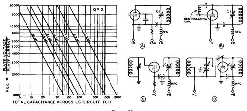
Figure 23 PLATE-TANK CIRCUIT ARRANGEMENTS
