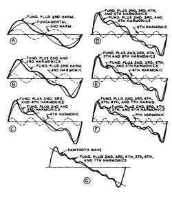
Figure 26 COMPOSITION OF A SAWTOOTH WAVE
