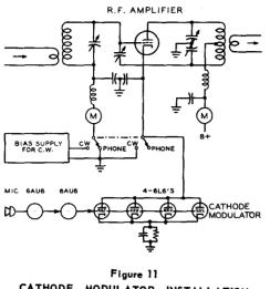
CATHODE MODULATOR INSTALLATION SHOWING PHONE-C.W. TRANSFER SWITCH
