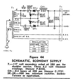
The schematic of a typical supply is shown in figure 46. Primary power source may be either 115 or 230 volts, the latter providing slightly better power supply regulation. The two transformer primaries are connected in series for 230 volt operation, or in parallel for 115 volt operation. In addition the primaries may be connected in series for halfvoltage operation on 115 volts as shown. The supply provides 750 volts at 400 ma. under this operating condition.
