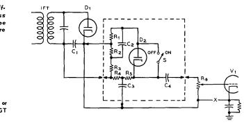
Figure 31 ALTERNATIVE NOISE LIMITER CIRCUIT
