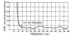
Figure 25 SWR CURVE FOR A 13.2 MC. DISCONE ANTENNA. SWR IS BELOW 1.5 TO 1 FROM 13.0 MC. TO 58 MC.
