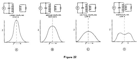
EFFECT OF COUPLING ON CIRCUIT IMPEDANCE AND Q
