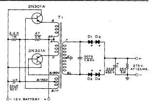
at 50 milliamperes, simultaneously). Both power units operate from a 12 volt primary source.
