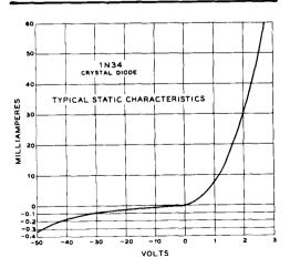
Figure 1A TYPICAL CHARACTERISTIC CURVE OF SEMI-CONDUCTOR DIODE
