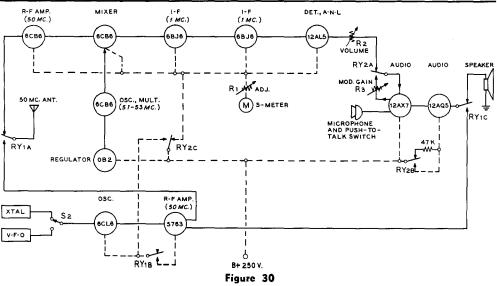
BLOCK DIAGRAM OF 10 WATT SIX METER TRANSCEIVER
