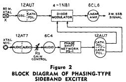
Only five tubes are required in this simple phasing-type sideband exciter. Audio system has sufficient gain to operate from crystal microphone.
