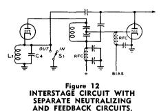
It is convenient, however, to separate these circuits so neutralization and feedback can be adjusted independently. Also, it may be desirable to be able to switch the feedback out of the circuit. For these reasons, the circuit shown in figure 12 is often used. Switch Si removes the feedback loop when it is closed.
