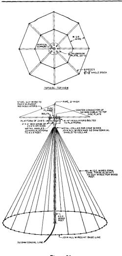
Figure 26 MECHANICAL CONSTRUCTION OF 20-METER DISCONE
