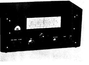
Figure 16 FRONT VIEW OF AMATEUR BAND RECEIVER 6-band receiver covers 80-6 meters, using TV turret for "front end." Mechanical filters provide optimum selectivity.
