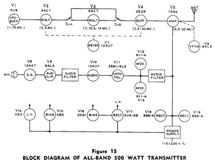
R-f section employs bandswitching exciter for coverage of 10, 15, 20, 40, and 80 meter bands. Variable frequency oscillator operates in 1.7 Mc. region to achieve maximum isolation. Tuning and antenna loading are aided by 6AL5 vacuum tube voltmeter monitoring output of amplifier stage. Low level speech clipping and filtering, combined with high level audio filter imports "punch" to phone signal, yet holds sidebands to a minimum. Single high voltage supply powers modulator and final amplifier.
