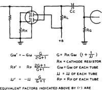
EQUIVALENT FACTORS INDICATED ABOVE BY (') ARE THOSE OBTAINED BY USING AN AMPLIFIER WITH A PAIR OF SIMILAR TUBE TYPES IN CIRCUIT SHOWN ABOVE.
