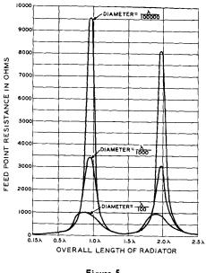
Figure 5 FEED POINT RESISTANCE OF A CENTER DRIVEN RADIATOR AS A FUNCTION OF PHYSICAL LENGTH IN TERMS OF FREE SPACE WAVELENGTH
