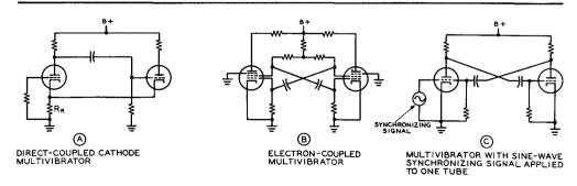
Figure 8 VARIOUS FORMS OF MULTIVIBRATOR CIRCUITS
