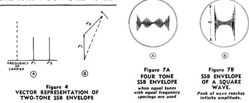
in amplitude modulation is of no practical value in SSB because the SSB r-f envelopes are so different than the audio envelopes. A heavily clipped wave approaches a square wave and a square wave gives a SSB envelope with peaks of infinite amplitude as shown in figure 7B.
