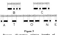
Diagram illustrating relative lengths of dashes and spaces referred to the duration of a dot. A dash is exactly equal in duration to three dots; spaces between parts of a letter equal one dot; those between letters, three dots; space between words, five dots. Note that a slight increase between two parts of a letter will make it sound like two letters.
