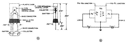
Figure 2A CUT-AWAY VIEW OF JUNCTION TRANSISTOR, SHOWING PHYSICAL ARRANGEMENT
