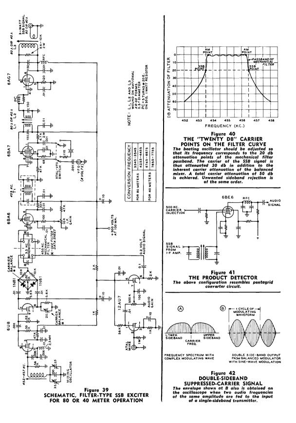
transformer is placed between the mixer stage and the 6AG7 output stage. A maximum signal of 3 watts may be obtained from the 6AG7 linear amplifier.
