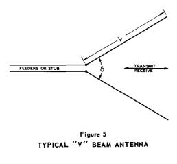
for a long wire. The reaction of one upon the other removes two of the four main lobes, and increases the other two in such a way as to form two lobes of still greater magnitude.
