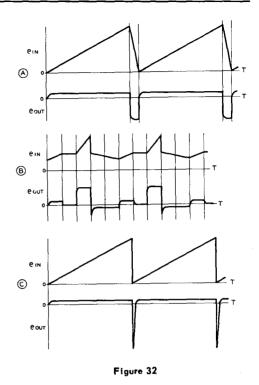
Differentiator outputs of short r-c circuits for various input voltage waveshapes. The output voltage is proportional to the rate of change of the input voltage.
