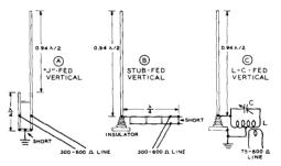
Figure 4 HALF-WAVE VERTICAL ANTENNA SHOW-ING ALTERNATIVE METHODS OF FEED
