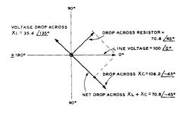
Figure 14 Graphical construction of the voltage drops associated with the series R-L-C circuit of figure 13.
