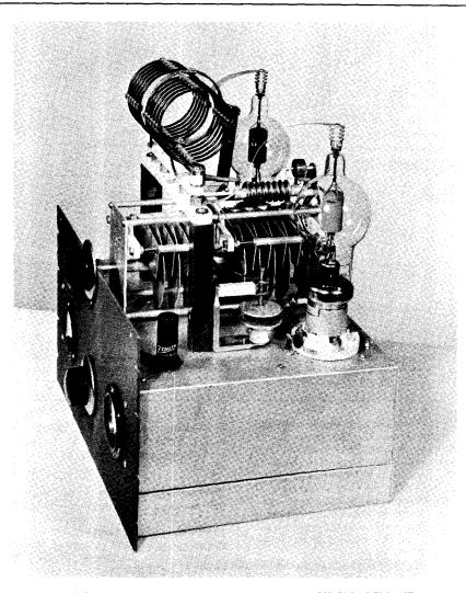
A PUSH-PULL 250-TH AMPLIFIER WITH TVI SHIELD REMOVED Use of harmonic filters in power leads and antenna circuit reduces radiation of TVI-producing harmonics of typical push-pull amplifier. Shielded enclosure completes harmonic reduction measures.
