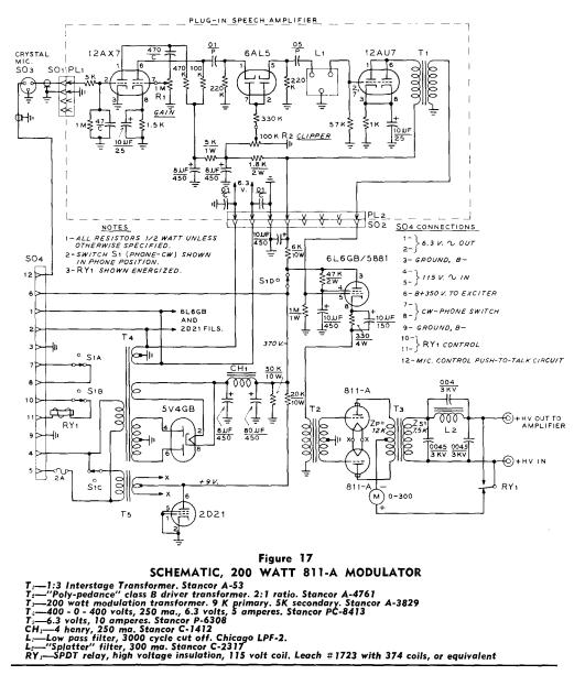
1250 volts, and only -4.5 volts is required for 1500 volt operation. Bias voltage may be obtained from flashlight batteries or other low impedance source.
