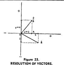
Any vector such as  $\dot{Z}$  may be resolved into two vectors, x and y, along the X- and Yaxes. If vectors are to be added, their respective x and y components may be added to find the x and y components of the resultant vector.
