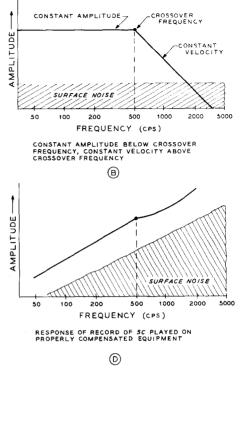
Figure 5 MODERN PHONOGRAPH RECORD EM-PLOYS CONSTANT AMPLITUDE CUT BELOW CROSSOVER POINT AND HIGH FREQUENCY PRE-EMPHASIS (BOOST) ABOVE CROSSOVER FREQUENCY.
