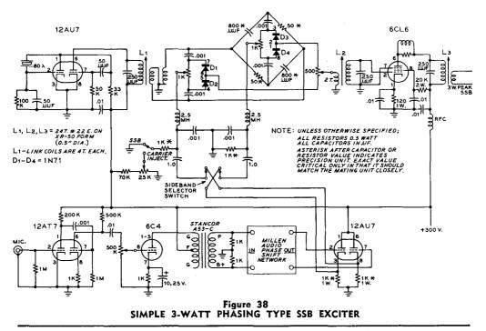
pole double-throw switch in the output circuit of the cathode follower permits sideband selection.
