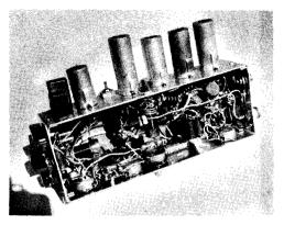
Figure 5 UNDER-CHASSIS VIEW OF SSB EXCITER
