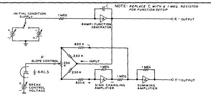
Figure 25 SIMPLIFIED DIAGRAM OF FUNCTIONAL GENERATOR TO APPROXIMATE NON-LINEAR FUNCTIONS.
