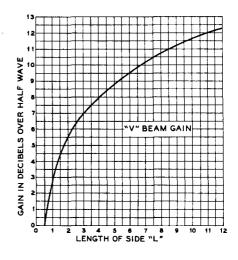
Figure 6 DIRECTIVE GAIN OF A "V" BEAM
