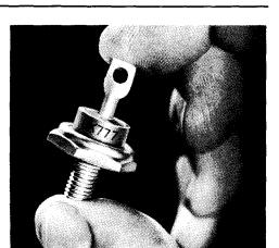
Figure 14 MINIATURE SEMI-CONDUCTOR TYPE RECTIFIER
