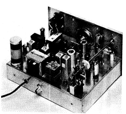
section of the unit occupies the center section of the chassis with the power supply directly behind it. To the right is the transmitter section with the variable frequency oscillator at the rear. Panel control of the oscillator is accomplished by an extension shaft and a flexible coupling. At the left of the chassis is the audio system.
