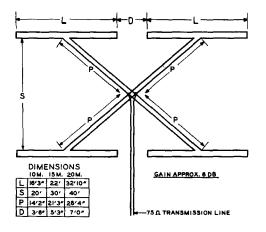
Figure 17 THE X-ARRAY FOR 28 MC., 21 MC., OR 14 MC.
