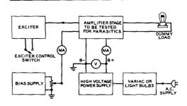
Figure 20 SUGGESTED TEST SETUP FOR PARASITIC TESTS
