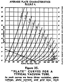
voltage, plate current, and grid bias. Each point on a grid bias line corresponds to the plate voltage and plate current represented by its position with respect to the X and Y axes. Those for other values of grid bias may be found by interpolation. The loadline shown in the lower left portion of the chart is explained in the text.
