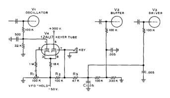
Figure 20 DIFFERENTIAL KEYER EMPLOYED IN "JOHNSON" TRANSMITTERS
