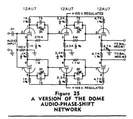
of the network and will show up as spurious emissions on the sideband signal, and also in the region of the rejected sideband. A lowpass 3500 cycle speech filter, such as the *Chicago Transformer Co. LPF-2* should be used ahead of this phase-shift network.
