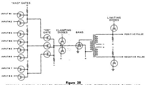
TYPICAL DIGITAL PACKAGE SHOWING INPUT AND OUTPUT DIODE GATES AND PULSE AMPLIFIER.
