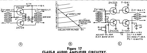
CLASS-B AUDIO AMPLIFIER CIRCUITRY. The common collector circuit of C permits the transistor to be bolted directly to the chassis for efficient heat transfer from the transistor case to the chassis.
