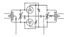
Figure 12 STANDARD CROSS-NEUTRALIZED PUSH-PULL TRIODE AMPLIFIER
