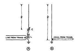
Figure 7 FEEDING A QUARTER-WAVE MARCONI ANTENNA
