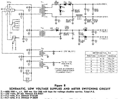
T<sub>1</sub>----6.3 volts, 6 a. Stancor P-3036 D<sub>1</sub>----y---Selenium rectifier, 100 ma., RMS input voltage: 175. Maximum peak inverse voltage: 495. Sarkes-Tarzian Model 108 D<sub>3</sub>--<sub>8</sub>-y---Selenium rectifier, 75 ma., RMS input voltage: 130. Sarkes-Tarzian Model 75 B<sub>1</sub>, B<sub>2</sub>---Srall 115-volt blower motor. St---2 pole, 6 position rotary switch. S0<sub>3</sub>---B prong octal socket (see figures 3 and 10)
