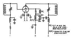
Figure 17 SCREEN PARASITIC SUPPRESSION CIR-CUIT FOR TETRODE TUBES
