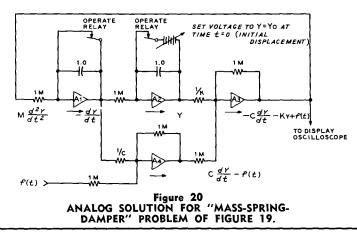
output of the summing amplifier (A3) to the input of the first as shown in figure 20 satisfies the equation.
