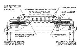
Figure 22 MECHANICAL FILTER FUNCTIONAL DIAGRAM
