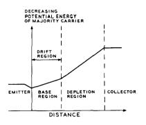
Figure 5 POTENTIAL ENERGY DIAGRAM FOR DRIFT TRANSISTOR (2N247)
