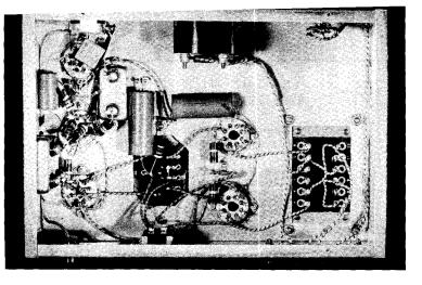
Figure 3 UNDERCHASSIS OF THE MODULATOR 6L6 Δ 4-connector plug is used for filaments and plate voltage to the speech amplifier, while a 6-wire terminal strip is used for the high-voltage connections and the transmitter-control switch.
