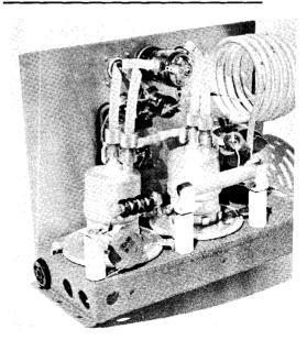
plate circuit of the amplifier. As a result, a very minimum of shielding and lead filtering is required with this amplifier even when 28 Mc. operation is desired. Placing the amplifier within the turtle-back of the automobile and the insertion of a low pass TV-filter in the coaxial antenna line reduces TVI-producing harmonics to such a low value that no interference is caused to a nearby television receiver tuned to a channel 2 signal of moderate strength.
