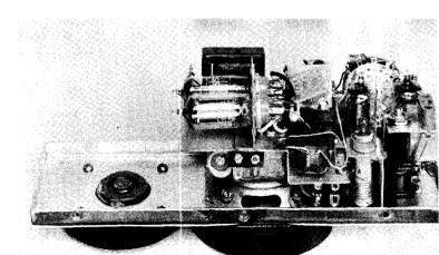
to the 144 Mc. doubler plate coil, L<sub>6</sub>. This coil is tuned for maximum output at 2 meters. After this preliminary alignment is completed the chassis of the transceiver may be placed in the case, along with the battery power pack.
