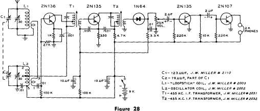
SCHEMATIC, TRANSISTORIZED BROADCAST BAND (500 - 1600 KC.) SUPERHETERO-DYNE RECEIVER.
