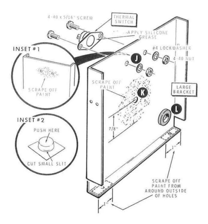
Locate the large bracket and scrape the paint from a 7/8" radius at hole K. Also scrape the paint from an area 1" from each end on the outside of the flange, and from around J, see inset #1.
