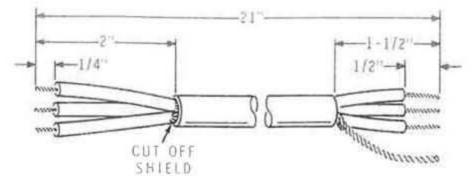
TAKING CARE NOT TO CUT THE OUTER SHIELD OF VERY THIN WIRES, REMOVE THE OUTER INSULATION.
