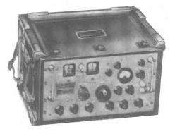
**R220/URR** RICEVITORE COLLINS MOTOROLA VHF da 20-230 Mc in 7 bande AM-FM-CW-FSK 110-220 V ac.
