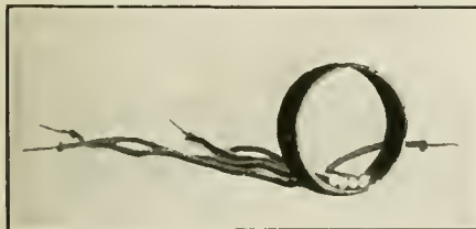
A New Form of Light-Sensitive or Selenium Cell. It Is Formed of Many Small Cells, All Held in a Brass Ring, Which Forms One Pole of the Circuit.
