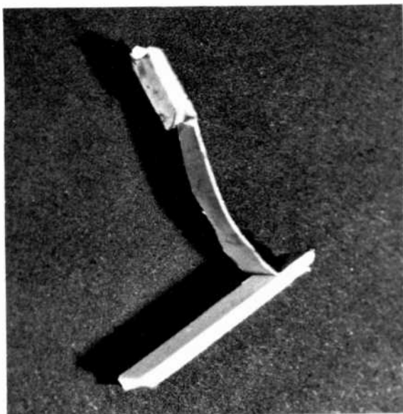
Fig. 2—Photograph of 200-mil wide substrate with electroplated handle.
