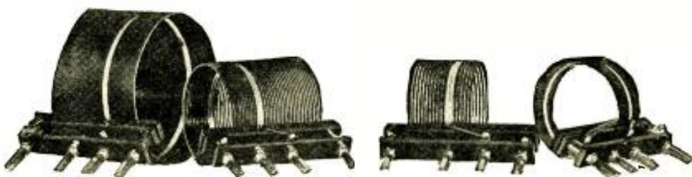
A set of the plug-in coils used in the adapter-receiver, with their standard interchangeable mountings. The space-wound wires are supported on an insulating film.
