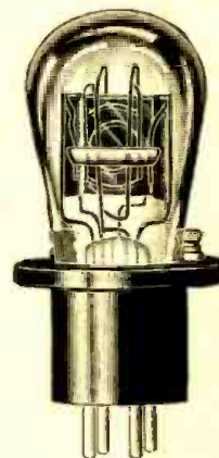
A.C. Adapter Tubes to convert battery sets into A.C. Electric sets—furnished for 226, 227, 171A.
