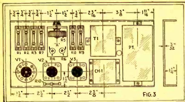
The layout of the upper side of the direct-coupled amplifier, which is made on a chassis of sheet aluminium, or other metal, shown in cross-section at the right of the drawing. Two strips of hard rubber are required to insulate parts from the chassis: one vertical, 3"x2", to carry R5 and J1 (if used); and one horizontal, 2 3/4"x2", supporting R4 and R6, as shown at A. In addition, it will be necessary to make up suitable metal clamps for use to support the by-pass condensers below the deck.
