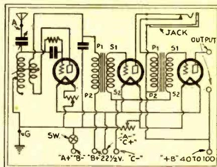
(Fig. Q.98) The "Model 52" regenerative 3-tube Crosley is also quite out of date, but may well be adapted to various needs, as an oscillator, "portable," etc.
