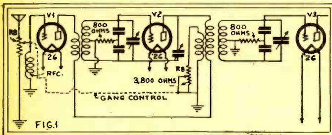
a dual volume control; one resistor is an aerial potentiometer, the other is across an R.F. absorption-circuit winding (Fig. 1). The arm of the latter resistor is fastened to the metal construction of the unit and, consequently, is grounded when mounted to the metal chassis; the other, coupled to the first by a strip of bakelite insulation, should be connected to the grid lead of the first R.F. tube.
