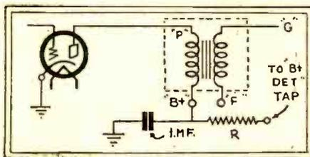
*The 1-mf. by-pass condenser shown above will often greatly improve the output of a set, particularly when its filtering action is aided by the use of R. An appropriate value for this resistor is 60,000 ohms.*
