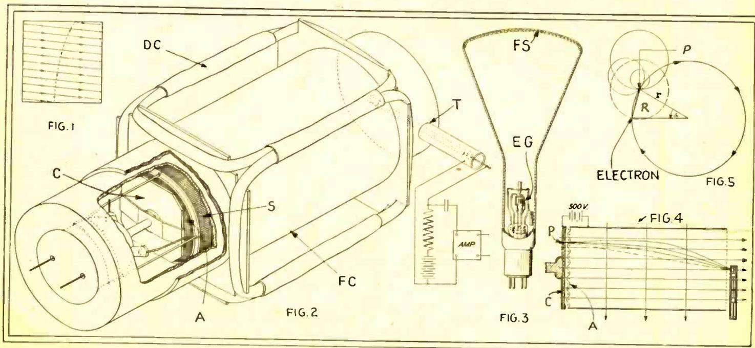
The magnetic scanning at the upper left assumes its shape as a resultant of two moving fields. The "dissector" of Fig. A is shown here internally in Fig. 2; and the "oscillite" of Fig. B in cross-section in Fig. 3. Fig. 4 illustrates the path of electrons from an illuminated point on the cathode; and Fig. 5 is an end-on view of their rotating motion. The object is to bring them all to the same point at the target.
