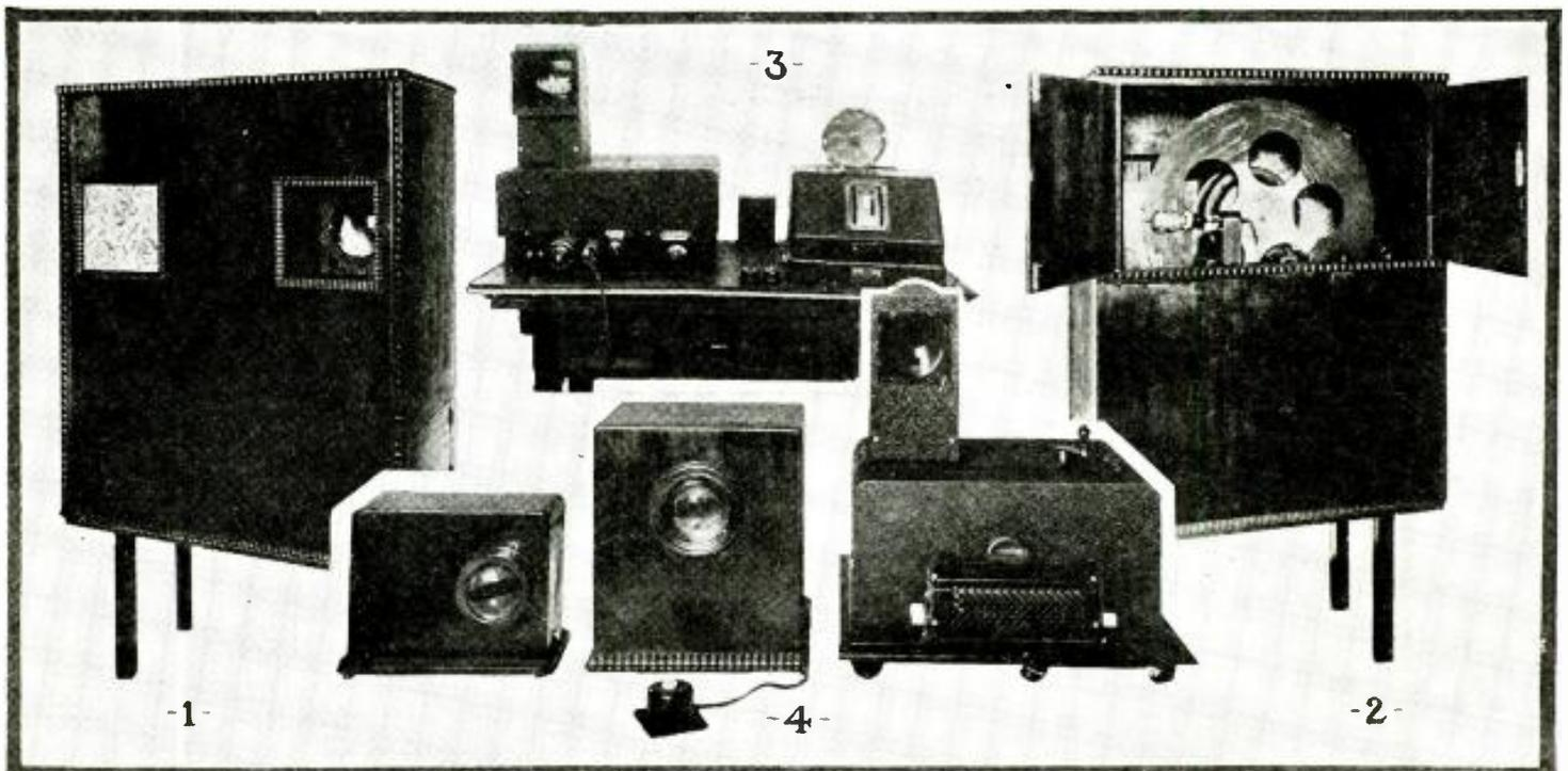
A group of televisions produced by the Telchor Company, of Berlin, which is developing the inventions of D. von Mihalý. The large sight-and-sound receiver shown at 1 is viewed from the rear at 2; it has a large disc, reproducing the image at the side in the window. At 3, a layout including a modern German broadcast receiver, with a television at its left; here the image is reflected upward into a "window." In the foreground at 4 are small televisions, one in the center with a speed control.
