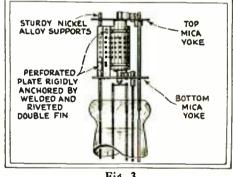
Fig. 3 The Arcturns "unitary" tube construction, pro-ducing a rigid, uniform assembly which makes characteristics permanent.
