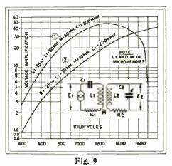
Curves obtained from a commercial autenna transformer; in (2), the primary is smaller and the coupling is looser. Note that the vertical scale is lonarithmic.
