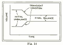
The result of unbalanced halves of the pushpull circuit. After a very short time, in which re- and de-generative actions occur, normalcy is reached.
