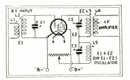
Mr. VanLeuven suggests the use of a dynatron frequency-changer, as shown above, instead of a separate oscillator, for experiment in superheterodyne circuits.
