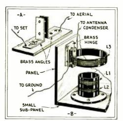
The antenna condenser of a short-wave set may be a standard small-capacity midget, or a pair of anales like those at A, though these are less easily adjusted. A method of coupling to the aerial with plug-in coils is shown at B. condenser.
