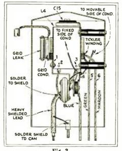
Fig. 3 Details of 1.4; the tickler winding, 5-6, does not appear on coils 1.2 and 1.3. The grid lead is shielded.
