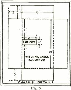
The chassis mounts every part of the beatfrequency oseillator; it is cut from a single sheet of metal, as shown, and bent to form a pan.
