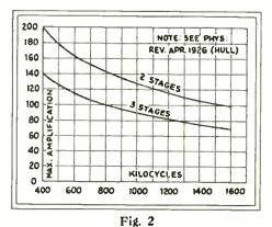
The theoretical limit of screen-grid amplification; on the basis of 1000 micromhos of mutual conductance, and .02-mmf. grid-plate capacity in the screen-grid tube.
