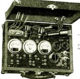
contains the same equipment as the "Model 700"; but the apparatus is arranged in a tray and installed in a slightly larger carrying case, with a space below the tray  $43_4$  hy  $61_4$  by  $133_4$  inches, which is suitable for carrying tools, spare tubes, etc. The tray is so contrived, that it may be taken out of the case and placed on the workbench.
