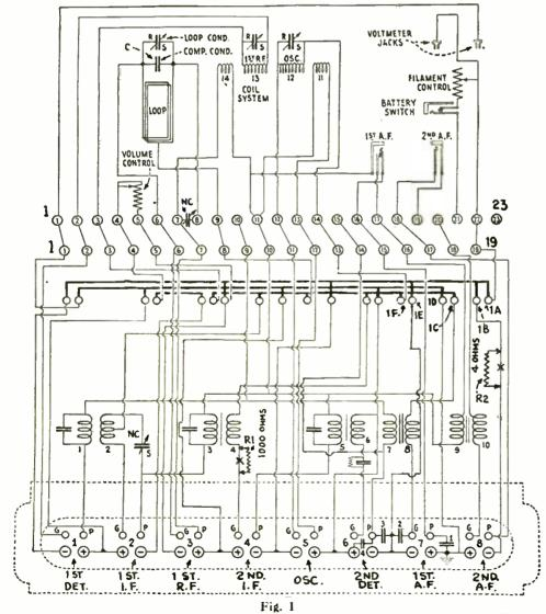
Schematic circuit of the "Radiola 28" (see also pape 653), showing needed changes. A "Type 934" Connectorald may be used externally, instead of opening the catacomb to introduce RL. The numbers of the "whisker" connections, 1-19, are stamped on the under side of the bakelite panel.
