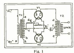
Fig. 1 The new familiar pushpull circuit, with its biasing resistor Rg un-bypassed, for reasons which are explained in the text.
