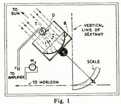
The principle of the radio sextant; it measures the angle between the sun and the harizon. The meter reads maximum when the image of the sun is concentrated on the perforation in the diaphraym D
