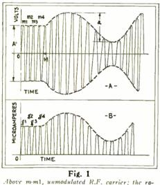
choose mm1, unmodulated K.P. carrier; the ratio u/A is the percentage of modulation. This wave is, theoretically, "detected" into the halfwave form below, where g-g1 is the rectified carrier.
