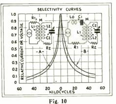
Selectivity curves at 1000 kc. of interstage coupler (A) and acrial coupler (B). The former has the high tube resistance K1, and the latter the high acrial capacity, in the primary circuit.
