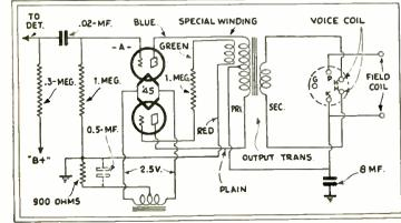
In Fada models "50" and "70," trouble may be found from open grid suppressors of the wire-wound type. If they are replaced with carbon resistors, the trouble is remedied.
