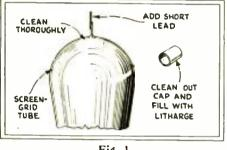
Fig. 1 The loosened cup of a screen-grid tube may be cemented back into place, quite satisfac-torily, in the manner shown.
