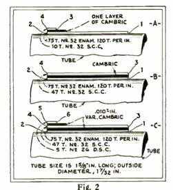
Specifications of I.F. transformers, in the following order: A, I.2; B, I.3; C, I.4-seconddetector, with feed-back coil having terminals 5 and 6.
