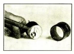
A coltractor, with its case removed, undergoing the operation described by Mr. Nothelfer, which gives access to the basic milliammeter unit,
