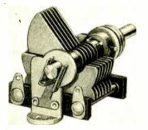
The new Hammarlund Junior Midline Short-Wave Condenser, capacity .0002 mfd. The rotor plates turn in a diameter of only 2 inches, while the total frame depth is only 15% inches. So this is an extremely compact condenser, made by one of the foremost condenser manufacturers in the world. It is our Model No. PR-H-20, made specially for us.
