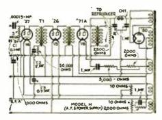
of R.F. amplification, making six tubes in all. Other details are as follows. There is in the antenna circuit a fixed .001-
