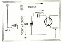
Mr. Pfeiffer cuts down the number of coils which it is necessary to plug in, with S.P.D.T. switch at No. 2. . In anti-capa an S.P.D.T. switch at No. 2. . . In anti-capacity switch on the panel might be more convenient.
