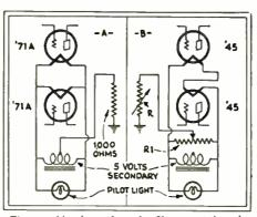
The combination of series-filament tubes in push-pull is not completely balanced; but the circuit tends to equalize the effect of differing grid biases.
