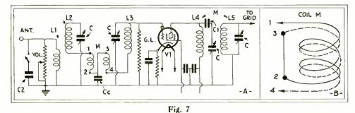
Details of a band-selector circuit, utilizing a combination of capacitative and inductive coupling in the antenna, together with mutual-inductance coupling in the interstage circuit. At least four tuned circuits, as shown, should precede an nutured amplifier. The detail of the first coupling coil M (left) is shown at B (right).
