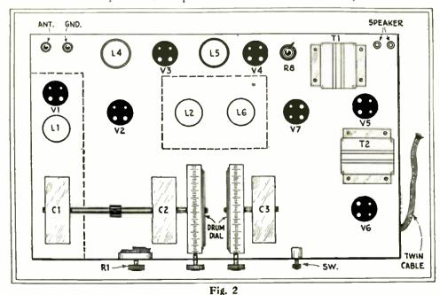
The layout used by Mr. Smith; the oscillator coupling is obtained between the fields of the two coils L2 and L6. The tubes V2, V3 and V7 have individual shields, as well as the coils L4 and L5.
