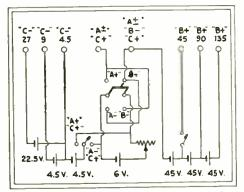
An arrangement of battery supplies for the service bench where D.C. receivers are generally in use. The switch adjusts for return of "B-," to ".1+" or ".4-."
