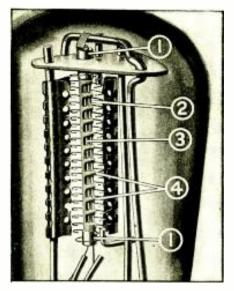
Fig. A The new De Forest cathode-heater construction—1, cathode tube: 2, 3, filament; 4, "fins."
