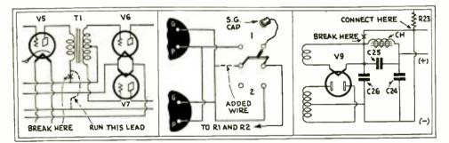
accordance with the diagram (Fig. 2) which failed to show one lead of the wiring. The grid conto show one lead of the wiring. The grid con-nections of the sockets should be connected to the
