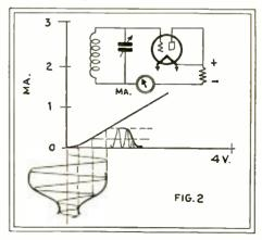
The characteristic operating curve of a "diode" detector (plate and filament joined).
