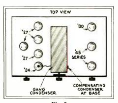
Fig. 5 Position of trimmer on Emerson chassis.
