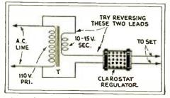
A step-down transformer T may be used to aid love line-valtage; a 0-150-volt A.C. meter will love line-valtage; a 0-150-volt .1.C. n show the proper connection.
