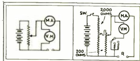
Figure 3, left. The voltmeter-ammeter method of measuring resistance.
