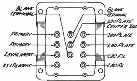
Power transformer terminal connections of the Model 99 Chassis.
