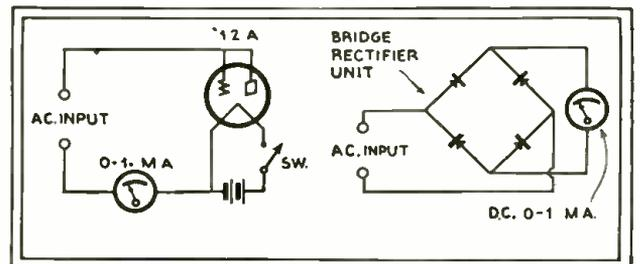
**Figure 8 left.** The use of the vacuum tube as a rectifier used for measuring A.C. voltages.
