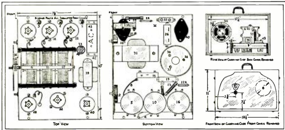
Figure 2, left and center. The complete layout of the parts is indicated. At the left, the top view, in the center, an under-side view. Figure 3, right. The position of the set after it is set in the carrying case. Above, rear; and below, front views.
