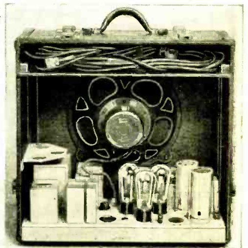
Left, the carrying case housing the projector; above, the case containing the amplifier and speaker in the W. E. portable sound system.
