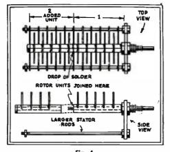
Fig. 4 Separately controlled condensers made by Pilot may be ganged as described here.
