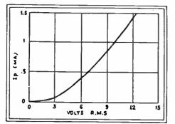
Fig. 3 A calibration curve of the V.T. voltmeter illustrated in Fig. 2. This meter will read voltages up to about 15, very easily. A 20 is used.
