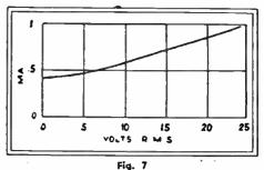
Calibration curve of the Reflex voltmeter illustrated in Fig. 6, to the left.
