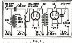
Fig. 11 A simple method of controlling volume on some 2-volt receivers. A change easily made.
