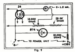
Connection of the voltmeter illustrated in Fig. 8 for use with an A.C. power pack. A pack may be made, or an old "B" eliminator used.
