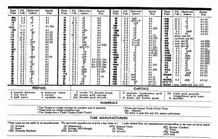
If no prefix is shown, the tube is a detector-amplifier.
