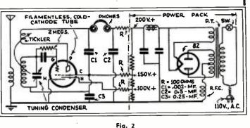
rig. 2 Schematic circuit of a one-tube receiver using the filamentless tube described in this article.
