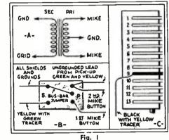
Fig. I At A, schematic and at B, pictorial view of the new microphone transformer. At C, the terminal block.
