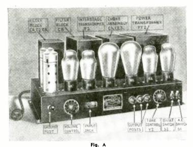
Photograph of the Coast-to-Coast 40-wait amplifier which employs Class AAA amplification. See Fig. 3, lower right.
