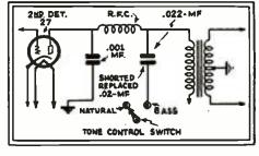
Fig. 8 Output detector circuit of the Majestic 20.
