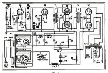
Fig. 3 Schematic circuit of the P. A. amplifier using two 59's feeding two 50's in the new, class AAA' circuit.
