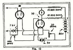
Complete schematic circuit of the Hoare V.T. voltmeter. This is a bridge arrangement using two tubes and a type 30 tube. Balance for zero read-ing of the meter in the circuit.
