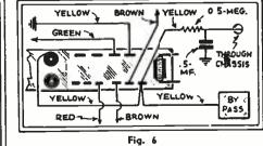
The resistor and condenser shown may be connected in the circuit to obtain better quality on low vol-ume in these receivers. This change was brought about by complaints that the set distorts on low volume. Incidentally, some of the changes recom-mended will also improve reception when used on "radio." Schematic circuit of the system without the pres-ence of the switches. This circuit shows the con-nections when the switches are thrown for microphone use.
