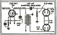
Fig. 7 Input arrangement of the Silver Marshall 36A.
