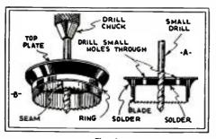
Fig. 1 This very versatile circle cutter may easily be made at home with the aid of the few parts specified by the author. It's handy, too.
