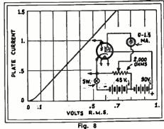
Calibration curve and circuit of a highly sensitive dynatron voltmeter. You may have to use an old type 24 for this circuit.
