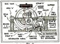
Fig. II A good "high powered" eliminator.
