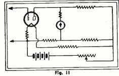
Fundamental circuit of the Hoare V.T. voltmeter. Details and circuit constants appear in the com-plete schematic circuit of Fig. 12, above.
