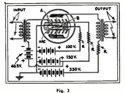
A theoretical circuit illustrating the use of the filamentless tube as an amplifier.
