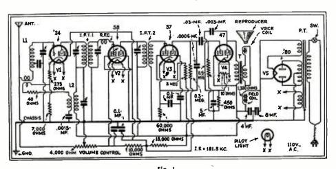
Fig. 1 Schematic circuit of the Crosley Book Case Receiver pictorially illustrated in Fig. A.
