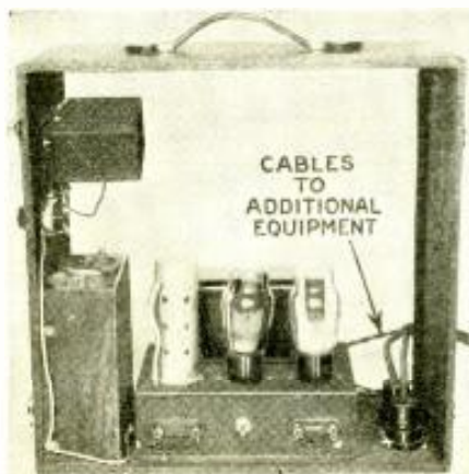
Close up of the Lafayette Dual Speaker Portable Amplifier. Along the left side are (top to bottom) mike coupling transformer, gain control, and mike batteries.
