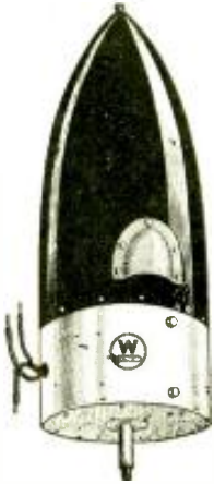
Outside View of Aircraft Generator
