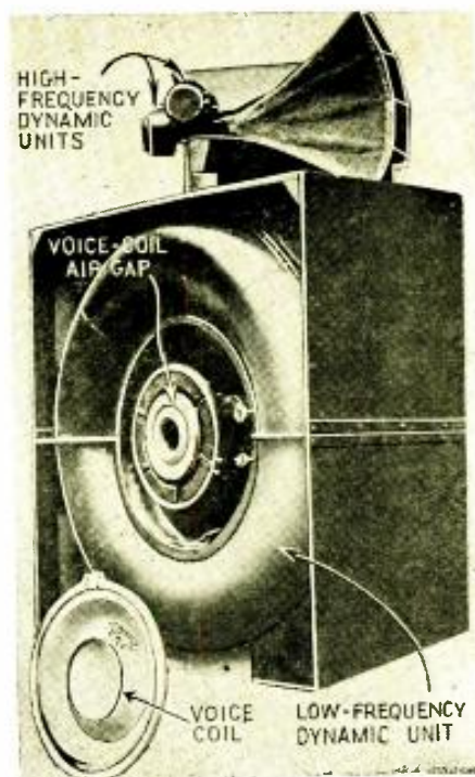
Fig. B, right Rear view. Note the very great diameter of the low-frequency voice coil. The reproducer assembly is designed to deliver an output of 100 db!
