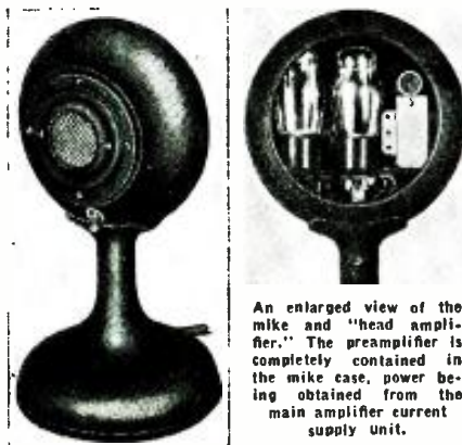
Fig. B The condenser microphone and preamplifier.
