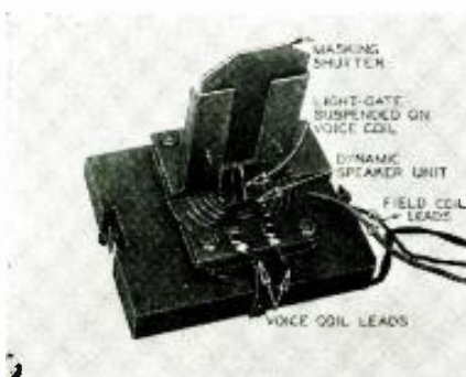
Fig. A Photograph of "light gate."
