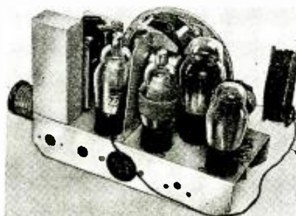
Rear view. Plug-in coil is shown at left.
