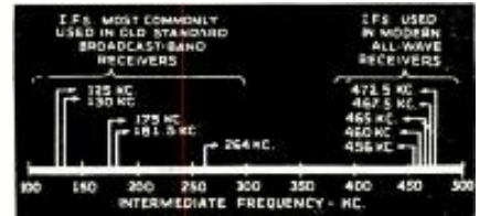
Fig. 1. This chart shows pictorially the positions of the various intermediate frequencies used in all-wave sets.
