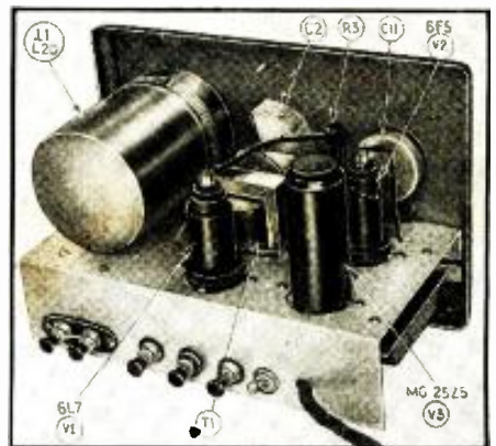
The rear of the chassis with tubes in place.
