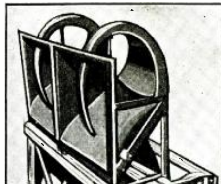
Fig. F. Twin exponential horns mounted on a movable tower for correcting defective distribution.
