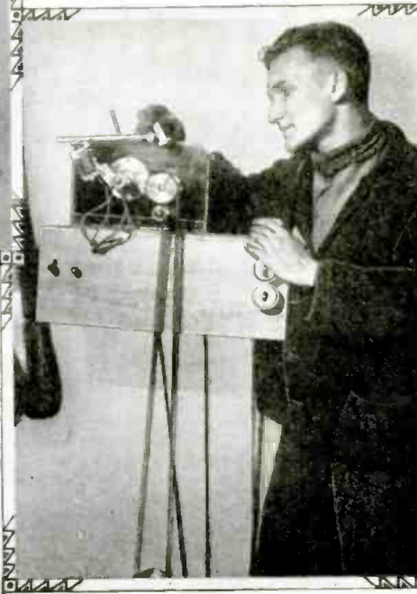
NEWEST TYPE KERR CELL. This was developed for television work by W. H. Peck. It is used to modulate the light beam; the bulb is almost entirely liquid-filled.
