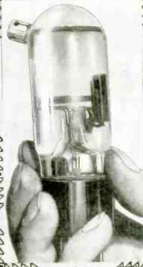
NEWEST TYPE KERR CELL. This was developed for television work by W. H. Peck. It is used to modulate the light beam; the bulb is almost entirely liquid-filled.
