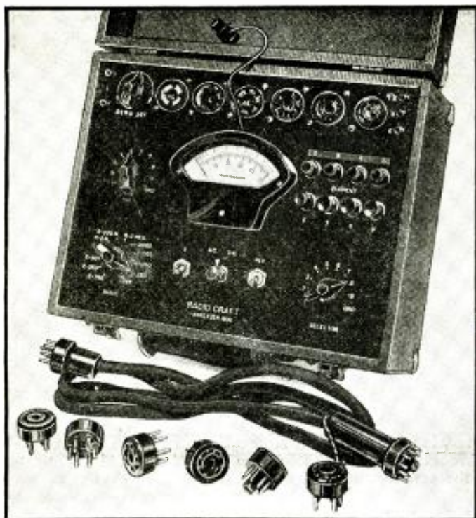
Fig. A. The complete analyzer—note the convenient layout of the controls; and the large meter.
