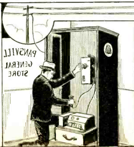
Fig. 1. The 3 steps. First the picture is taken, then developed; second, it is sent over the line; and third, received (as shown in Fig. D) at the newspaper office.
