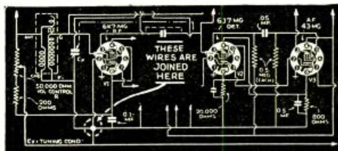
Fig. 1. A slight change is necessary in the circuit of the "Lazyman 4".
