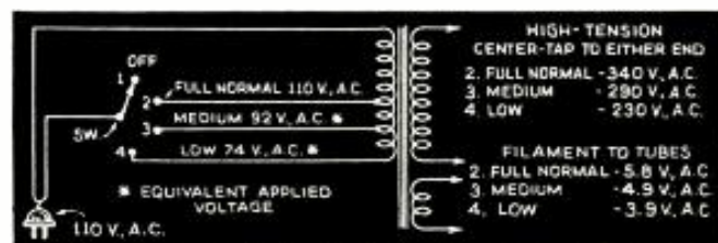
The transformer taps effect the current saving by reducing tube voltage.
