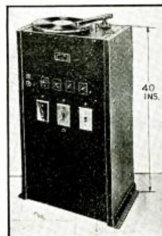
Panel amplifier. This 50-W. set-up will drive 50 dynamics. (1336)
