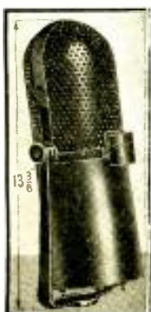
Fig. A. The completely-assembled view, left, of the new directional-type ribbon microphone shows it to be more than 1 ft. long. The lower-half of the case encloses the rod-aligned labyrinth sections (see view at right).
