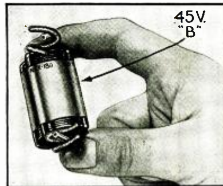
Fig. A. The appearance of the complete layerbuilt battery. The comparative size can be seen against the hand.
