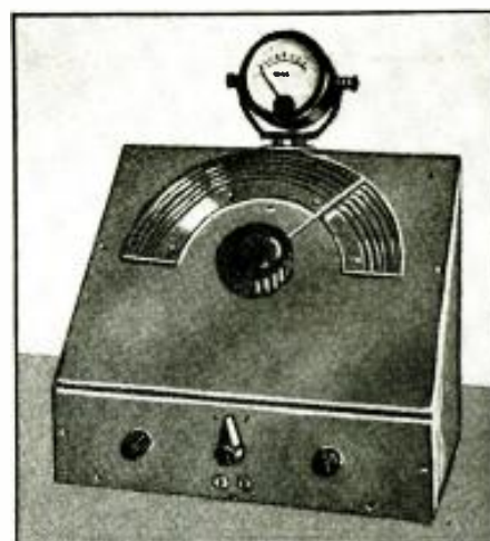
Fig. A. A new French bridge capacity meter.
