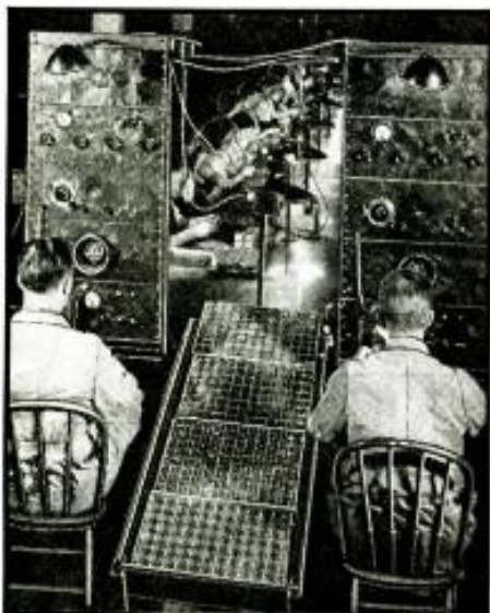
Photo courtesy Aladdin Radio Industries, Inc. Cathode-ray tubes are now being used in checking R.F. and I.F. coils in the factory of a prominent coil manufacturer. Much closer tolerances are made possible by this procedure because of the high sensitivity and lack of inertia in the C.R. tube.
