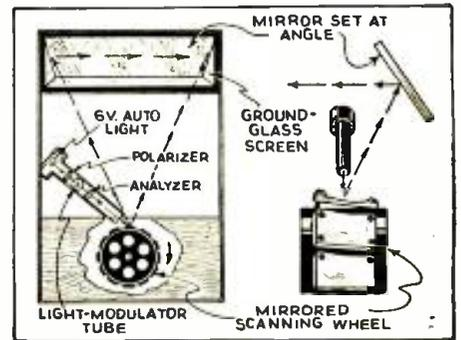
Fig. 1. Televised "copy" is transmitted via radio or wire. The receiver translates these impulses into light rays that are projected onto a mirror (screen).
