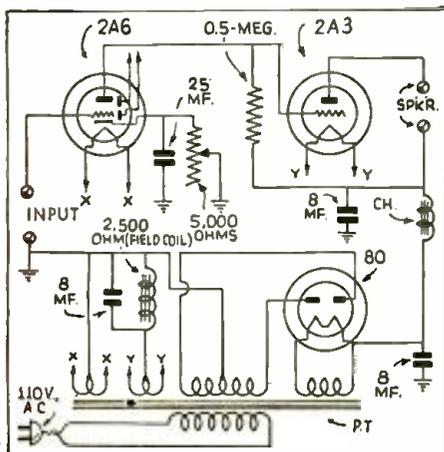
Fig. 1. The basic circuit of the D.C. amplifier.
