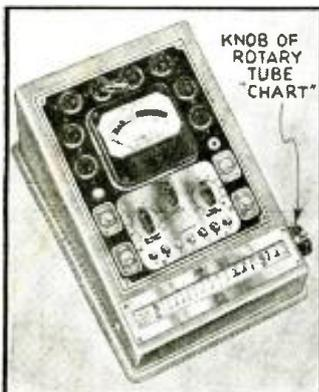
Modern tube checker includes built-in tube listing. (1423)
