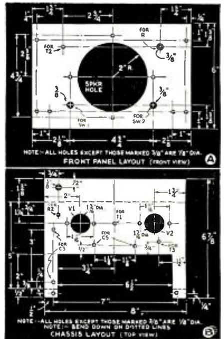
Fig. 4. Specifications of front panel and chassis.
