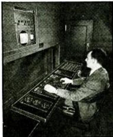
Left—the Television Traffic Man, watching the action in the studio, monitors the program on the Kinescope above the window. A breast microphone connects directly with . . . Right—the Iconoscope Camera Man, who is here shown putting Miss Hildegarda "on the air" via NBC-RCA at Radio City.
