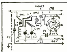
Switch Sw.2 is here shown properly wired-up to permit disconnecting L2 for making coil tests. The original circuit is Fig. 2 on pg. 18 of July, 1937 Radio-Craft.
