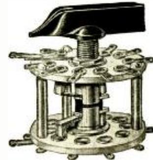
These switches can be made with any number of contact points up to fifteen, shorting or non-shorting, can be furnished with suitable insulation for metal panels, ganged in two or more decks, 1/4" shaft, single hole mounting. Ideally suited for band switching, high resistance voltmeters, multi-range instruments, etc.
