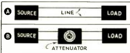
Fig. 1. Matching load to source with attenuator.
