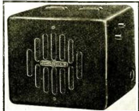
G.E. Model FA-60, in housing. The FA-61 differs in having a tone control, as shown in Fig. 1, with a knob at the lower-right of the grille, which also bears the letters "GE" in monogram. Speaker cover is held on by snap fasteners; 7 self-tapping screws secure chassis.
