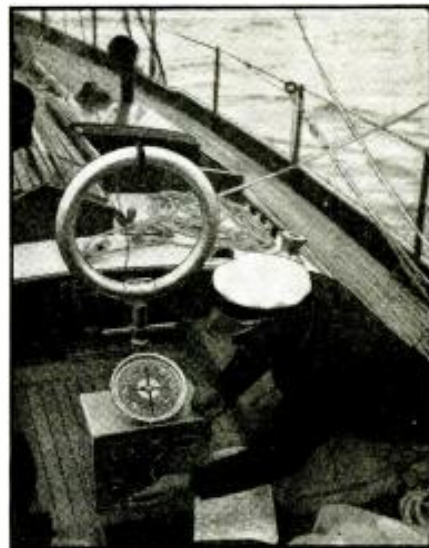
Fig. D. A Gloucester fisherman is here shown using a commercial make of marine radio direction finder. The position of a school of fish is charted for future reference by the use of this Bloodwell direction finder. Various lighthouses constantly broadcast (as part of their regular routine) a dot-dash signal. The direction of 2 or more of these houses is located (with the “finder”) and spotted on a chart. The point of intersection of straight lines drawn through these spots indicates the position of the ship and hence the school of fish; this prevents wasting hours in a search (on the next fishing trip) covering many miles.
