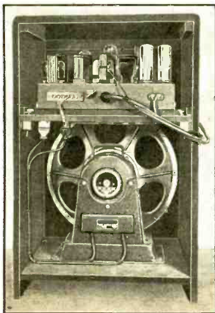
Fig. C. View inside the cabinet showing the location of the amplifier and speaker. As shown in Fig. 1A (page 402) the volume control on the amplifier is foot-operated, thus providing a "swell" pedal similar to that of an organ. This electric piano duplicates the acoustic characteristics of the mechanical piano which has a sounding board.
