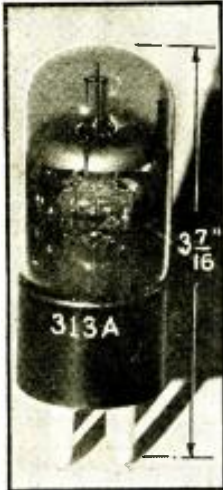
Fig. C 313A—cold-cathode gas-filled multi-purpose tube. It may be used as a relay, voltage regulator, or rectifier.
