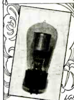
Helium Rectifier, 250 ma. Output for "A" Eliminators About 1925-6.
