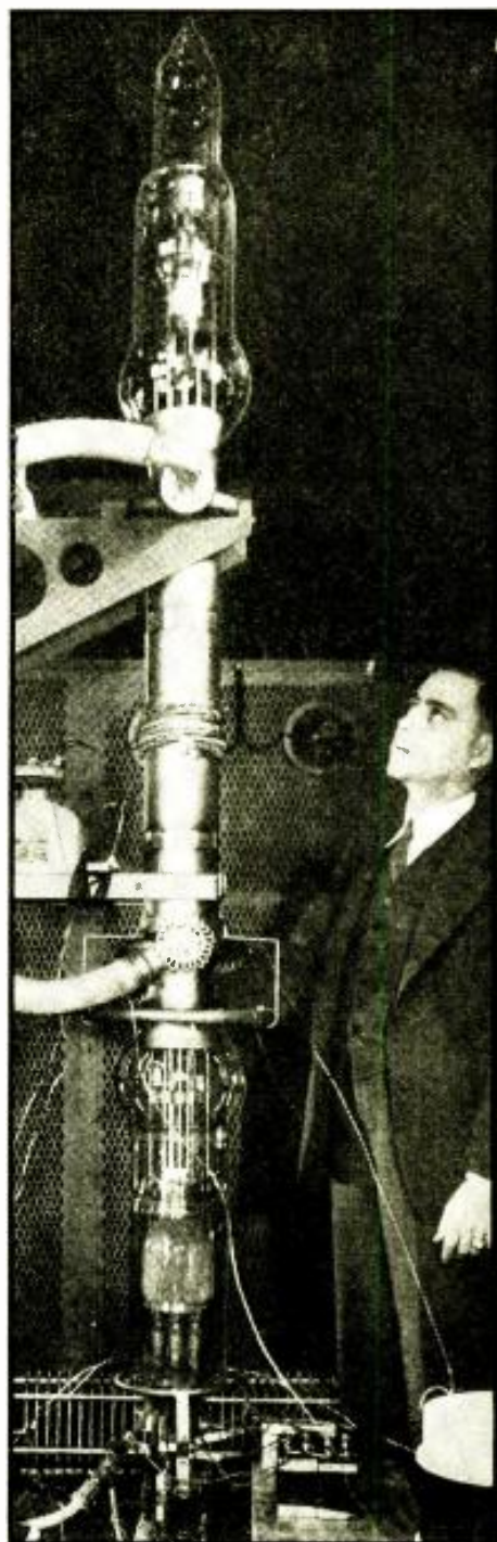
Fig. D. 1938's transmitter tube contribution to the electronic field, a 250,000-W. water-cooled giant.
