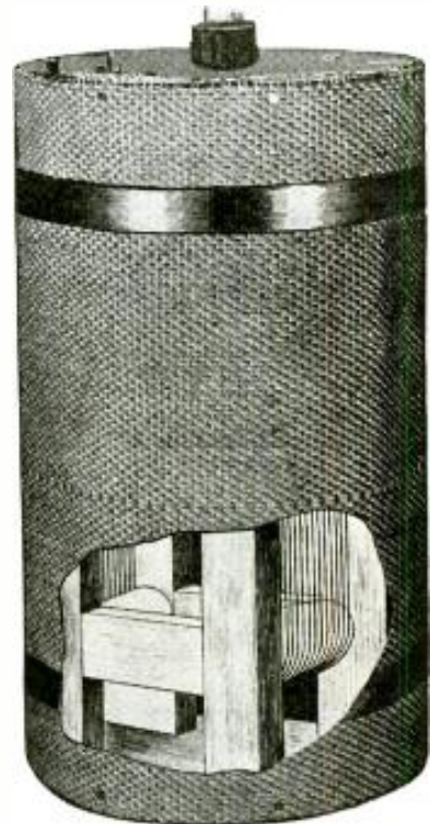
A shield around the loop stops static.
