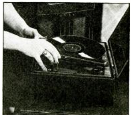
New wireless record player by Wholesale Radio Service Co. rounds out the famed Lafayette line. New unit sends modulated 1,200 kc. carrier; provides mike plug, too.
