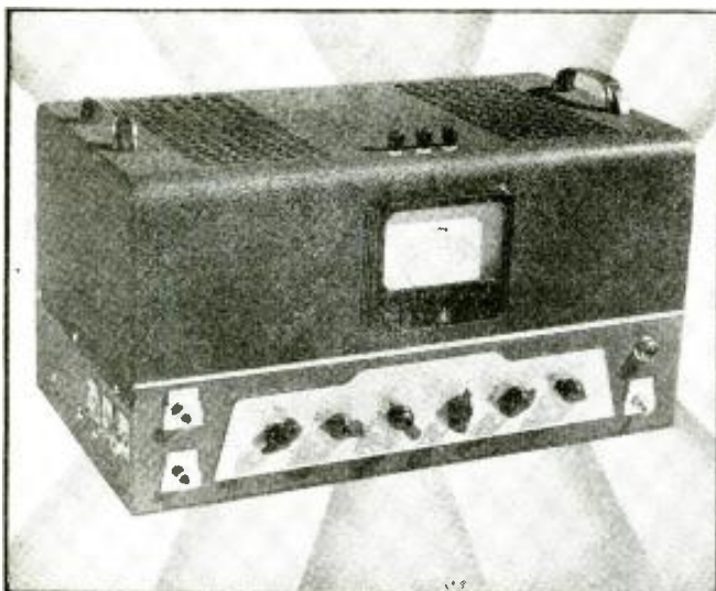
The complete, modern, Audio-Spectrum-Controlled Amplifier for Recording and Playback. The front panel controls from left to right are: plug-in jacks for 2 microphones, channel No. 1 voice-coil control, channel No. 2 voice-coil control, low-pass control, band-pass control, high-pass control, all-pass control, master switch and above it, the pilot light. Decibel-voltmeter posts are atop case.
