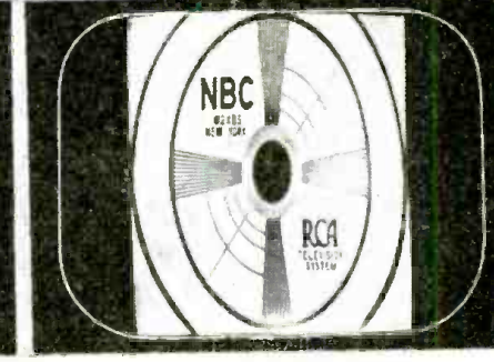
Fig. 10—INCORRECT WIDTH To correct—Adjust width control (screwdriver adjustment) for correct width of image.
