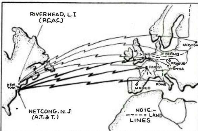
Radio circuits are shown solid; land lines are dotted. The A.T.&T. station at Netcong, N. J., has radio circuits to London and Paris only. The remainder of Europe is contacted by land lines. The R.C.A.C. station in Riverhead, L. I., has radio circuits to all the capitals of Europe.
