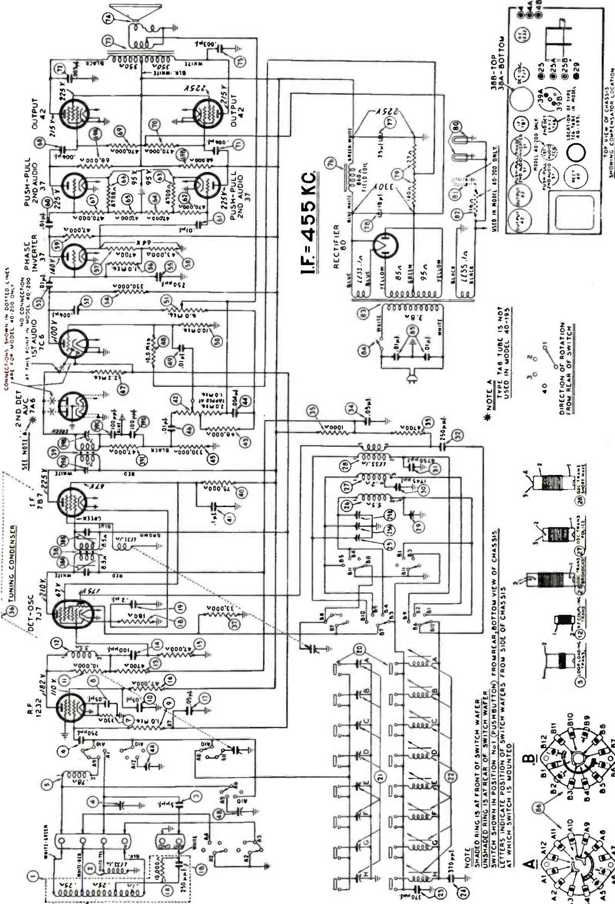
The voltages indicated were measured with a Philco Model 027 Voltmeter (1000 ohms per volt) — Power supply 115 volts, 60 cycle — Volume control minimum — No signal being received — Range switch "Bridge"
