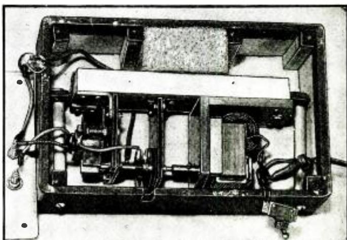
Fig. A. Inside view of the instrument showing the method of suspension inside the case.
