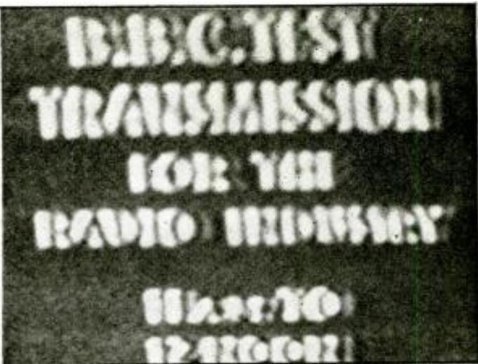
**Fig. 3.** This photograph depicts effects similar to those shown in Fig. 2, these are incorrect tuning of the oscillator, and low I.F.-circuit frequency response.
