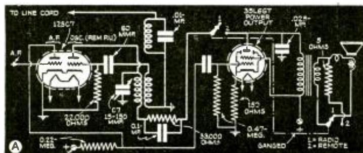
Fig. 2. New circuit features of (A) RCA Model 5X5; (B) Belmont Model 677.
