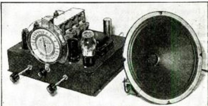
ables them to adjust the attenuation of the "highs" to suit their individual requirements. It should be noted that the on-off switch is an integral part of the tone control. This permits a relatively permanent setting of the volume control which is not disturbed by the turning on or off of the receiver.
