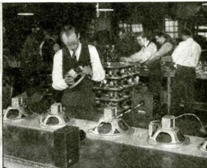
These photos illustrate but 2 of the thousands of industrial applications for photoelectric equipment. The illustration at the left shows photoelectric equipment used to assure the safety of the operator of a heavy punch-press. The illustration at the right shows the same photoelectric equipment, here used to count radio speakers as they pass along on an endless belt.
