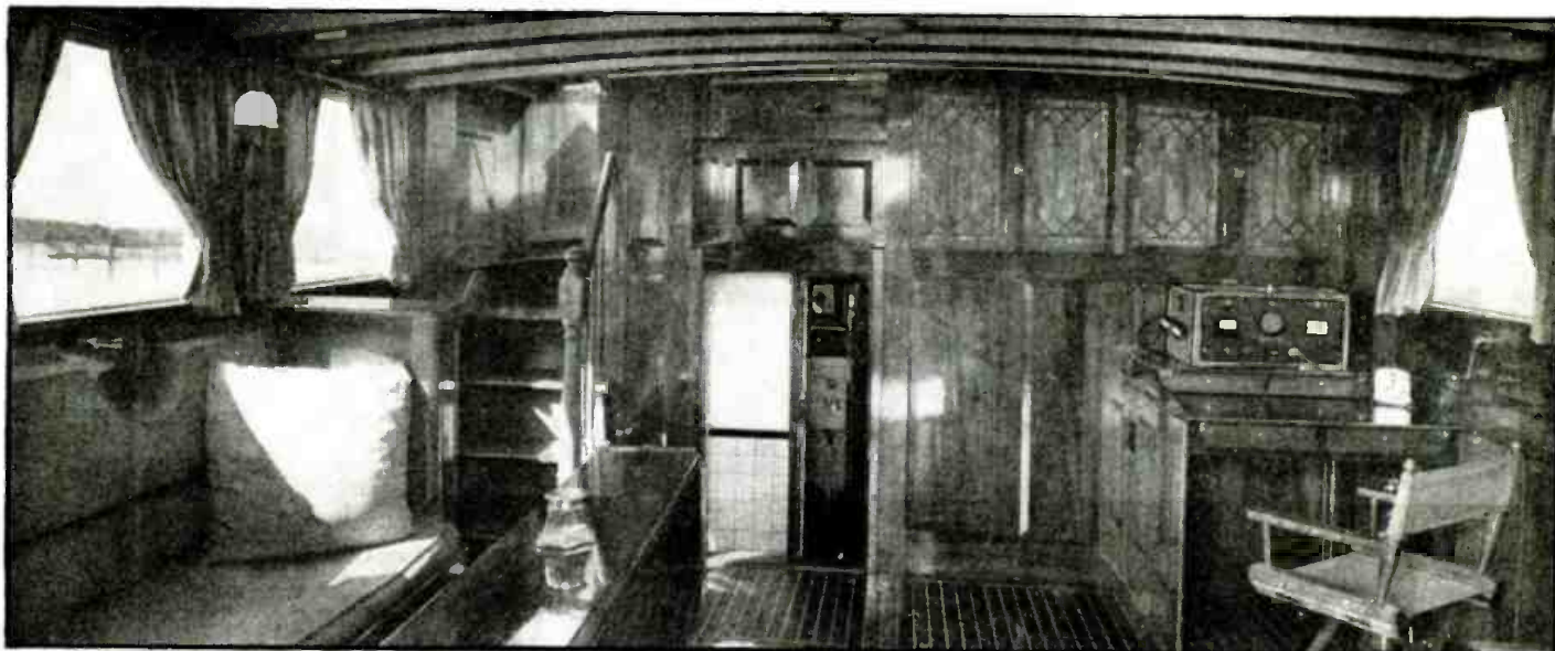
Fig. 4. A 25-watt Marinephone installed aboard the yacht V'entra . It serves to emphasize the importance of neatness in marine radio telephone installations.
