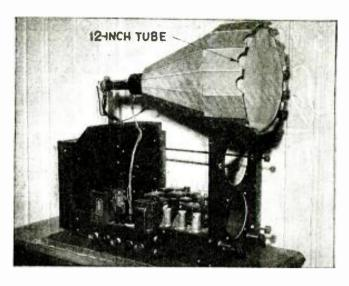
the failure of the supply. Look first to the 2X2 rectifier; then cheek the 2 filter condensers for leakage; and finally, cheek the voltage divider resistors for breakdown.
