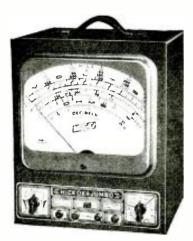
TS main feature is the display, 914-inch rectangular meter. Its ranges are as follows: A.C. and D.C. Volts, 0/10/50/250/especially handy for sensitive measurements; D.C. milliamperes, 0/5/50/500; ohms, 0.05/30 (8 ohms mid-scale), 0.5, 10,000 (150 ohms mid-scale), 50/1 megohm (15,000 ohms mid-scale), and 500/10 megohms (150,000 ohms mid-scale); decibels. -10 to +15, 29, 43. Output, 0/10 50/250 500/2,500. This range incorporates a blocking condenser.
