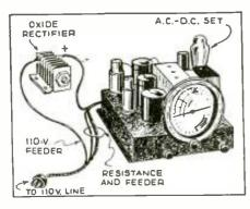
is properly connected as to polarity; rectifier gets "just warm." An old dry-disc rectifier from a trickle charger, connected as shown, will usually eliminate about 90% of the difficulty.
