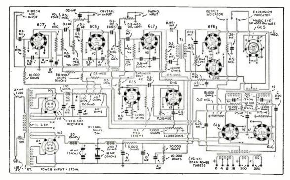
Circuit Diagram of An Anti-Howl Amplifier Described In The July, 1936 issue of Radio-Craft. The value and rating of resistor R in the voltage divider is given here (it was not given in the original presentation).
