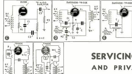
Fig. 7. Basic detection circuits. (A) Triode gridleakand-condenser detector. (B) Triode grid-bias detector. (C) Diode detection and A.V.C. (D) Duplex duodiode-triode tube (detector, and A.F. amplifier). (E) Diode-biased detector, using duplex duodiodetriode. (F) Dual diode detector and delayed A.V.C.
