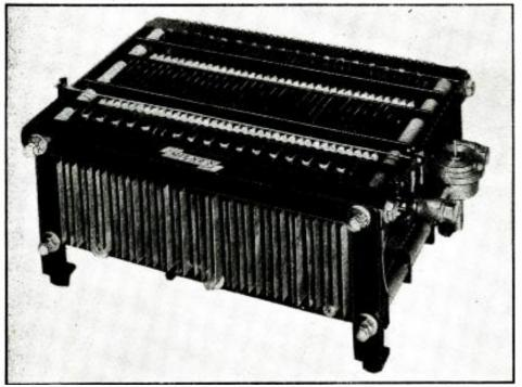
The Milnes converter-type Thermoelectric Generator is here shown with cover removed. It weighs 20 lbs., measures 12½ x 11 x 7 ins. high, and in American money would be priced at about \$20. It delivers 1 ampere at 2 Y. as "A" supply; and 2 amperes at 2 Y. to a converter, the output of which is 10 to 15 ma. at 120 V. for "B" supply; "C" is via a voltage divider. Cost to operate, only 2/3-cent per hour!
