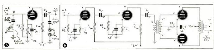
Fig. 5. Use of phono pickup for aural examination of A.F. amplifier stages. Fig. 6. Basic cascade (multi-stage) A.F. amplifier circuit with push-pull audio-output stage.
