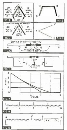
The various figures shown above detail the mechanical and electrical principles involved in the thermocouple, and the Milnes thermopile. Figure 4 is used to aid analysis of Fig. 9. In Fig. 7 is a graph which illustrates the watts output of the Milnes Thermoelectric Generator.
