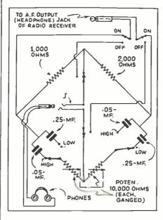
"birdies" to be eliminated (phased-out) during C.W. and phone reception; in fact, gives T.R.F. receivers the advantage in this respect ordinarily afforded only in superhets. with I.F.-circuit quartz crystals.
