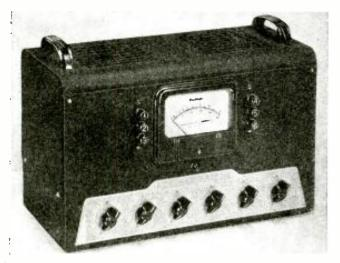
Fig. 1. The front-view photo of the completed hi-fi recording - playback sound amplifier, showing the cover in place; the various controls are identified as follows: pushbuttons (a left of the decibel meter, top to bottom)—Playback, Dialogue Filter, Record; (right) 0 Db., +20 Db., +30 Db. Bottom row of controls (left to right)—Mikes Nos. I & 2, Playback, Master Gain, H.F. & L.F. Controls.
