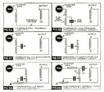
In the group, at left, of related diagrams—a circuit 'tamily'—are shown the circuit variations by means of which various arrangements for feedback produce changes in frequency response. While there may be a strong tendency by experimenters to construct this amplifier of junkbox parts, it is strongly recommended that the special output and power transformers be employed. (To avoid undue electrostatic and electromagnetic hum pick-up, precautions should be taken in wiring the input circuit.)
