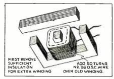
windings for pentodes such as 2A5 or 42; (2) pri. and sec. in parallel for power tubes, 45 or 2A3. Note: phase-out pri. and sec. to ensure against bucking one winding with other before paralleling them. The above combinations give 3 impedances; i.e., (1) primary winding, (2) secondary winding, and (3) pri. and sec. in parallel. The impedance varies with the ratio of transformer used.
