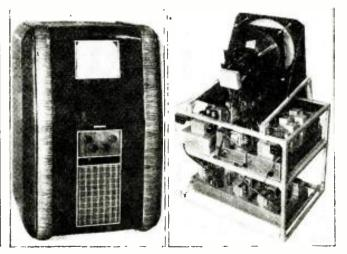
Last month Radio-Craft received from Allocchio Bacchini & Co. (Milan) these illustrations of the newest in Italian television equipment. The compact arrangement evident in the exterior view is explained by reference to the Interior photo at right. The arrangement of the coils for magnetic deflection eliminates astigmatism.
