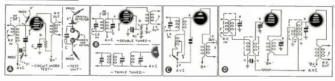
Fig. 8. Basic R.F. and I.F. circuits. (A) Basic R.F. pentode amplifier. (B) Basic I.F. amplifiers. (C) I.F. amplifier with adjustable transformer coupling. Position I = minimum selectivity; position 3 = maximum selectivity. (D) Bandpass T.R.F. amplifier.
