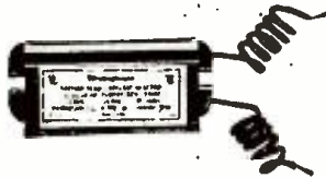
Fig. E. Fluorescent single-lamp ballast.
