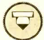
Shaft position in knob requiring 1/32" flat.
