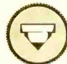
Shaft position in knob requiring 3/32" flat.
