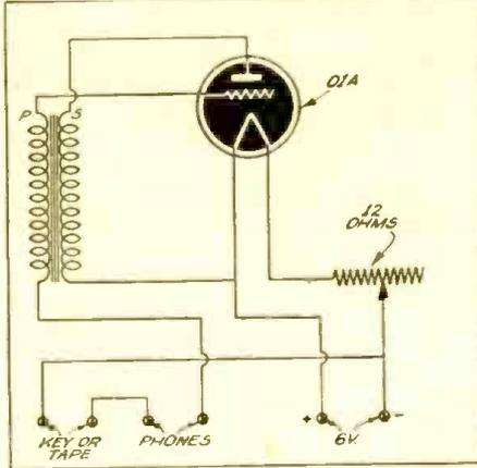
Here's a simple circuit for a code practice oscillator, sent by Mac Craighill, Box 308, Leesburg, Va. This oscillator can be built at slight cost; the transformer may be a 3 to 1 audio type. Rheostat regulates the tone.
