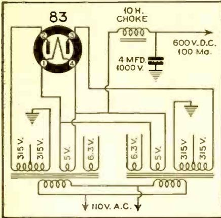
The diagram above, suggested by Harold Held, 57 Clark Street, Paterson, New Jersey, shows a simple way to obtain high voltage for transmitters, etc. Two receiver type power transformers are connected in parallel.
