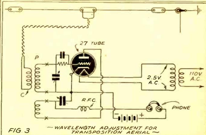
be coupled to the receiver or to the transmitter.
