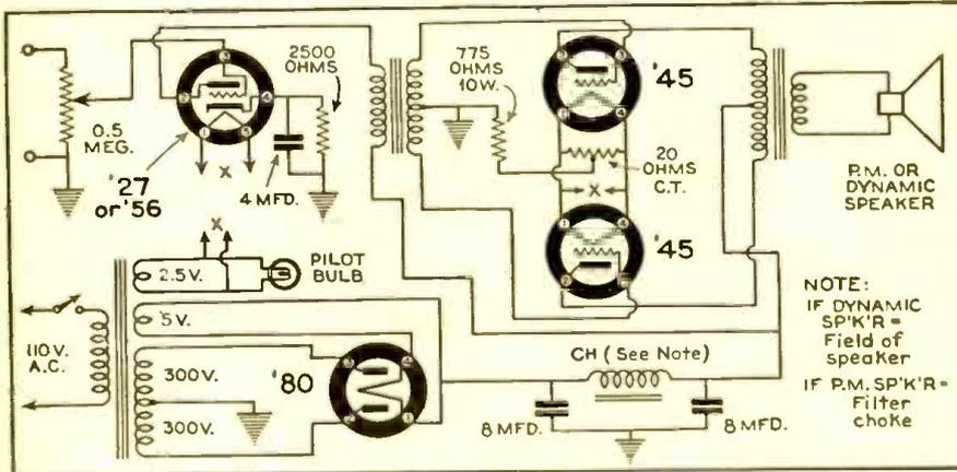
This 8-watt audio amplifier circuit was sent by D. McBride, Box 338, New Market, Ont., Can. This amplifier can be used to provide greater volume for a code practice oscillator, etc. Using midget transformers a very compact unit can be built; with a suitable pre-amplifier a good P. A. system can be assembled.
