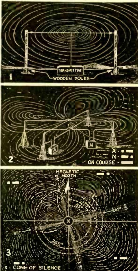
Figs. 1, 2, & 3.—Diagrams above show how radio waves spread out from a transmitter; also how A and N code signals are radiated.
