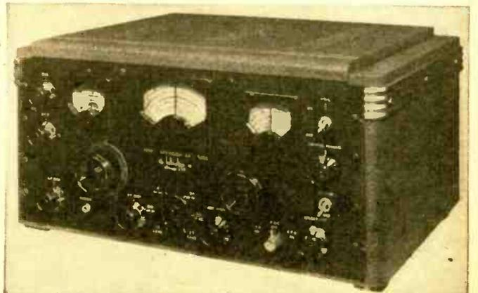
The new 1942 Model of Hallicrafters Communications Receiver, known as the "Skyrider 32" is here illustrated. All of the necessary controls for extremely selective tuning are provided.
