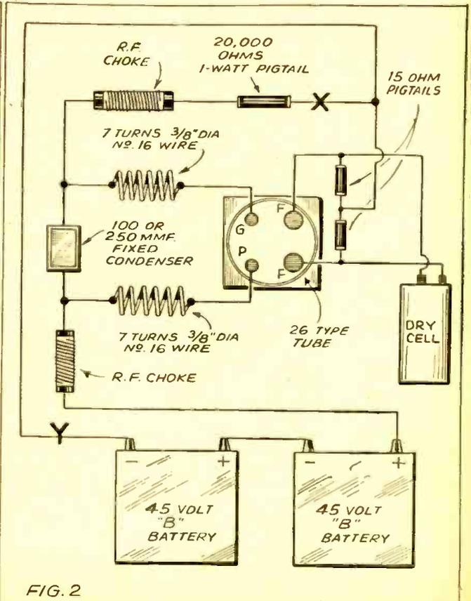
use D.C. on the plate and not to use an aerial on the set. By opening or closing the spring windings of the coils, the wavelength can be adjusted to any desired value.
