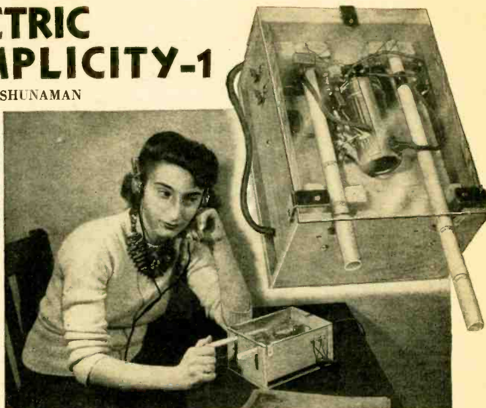
Tuning-up the all-electric model. The control being adjusted is the antenna tuner; the other one is the R.F. plate unit. Ventilation slots at the bottom of the receiver are easily discerned. Note glass cover on receiver.
