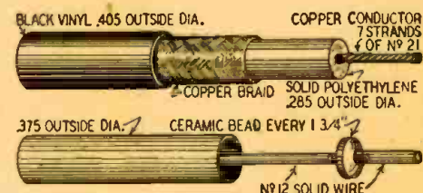
Fig. 6—Two types of popular co-axial cable.
