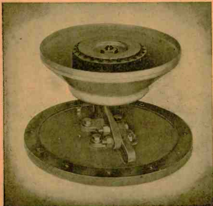
Photo A—Magnetostriction transducer used in underwater equipment.
