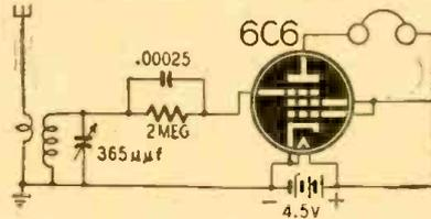
the suppressor as the control grid. In this way, the set works with only 4.5 volts on the various elements.
