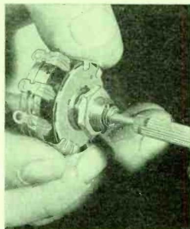
in conjunction with an assortment of flatted, round, knurled, and double-flatted shafts. The tip of the shaft slips into the hole in the control bushing until the keyway is engaged, whereupon a sharp blow on the end of the shaft, or hitting the shaft on a hard surface, drives the shaft securely into place.
