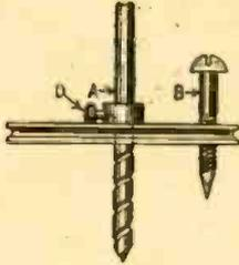
ened to hold it in position. A small bolt, selected to make a tight fit in one of the holes near the outer rim of the pulley, is ground to a triangular point for cutting. One nut is run up on the bolt before it is inserted in the hole and another is run up from the bottom to hold the bolt in place. The length of the bolt can be adjusted by changing the position of the two nuts. If a larger pulley is available, the bolt may be
