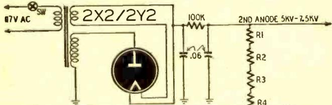
Fig. 2—High-voltage cathode-ray tube supply.
