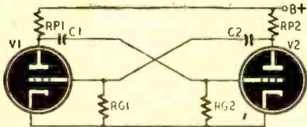
Fig. 1—The standard multivibrator circuit, consists of a 2-stage amplifier with the output of V2 fed back into the grid of V1. Due to the phase reversal of 180 degrees in each stage, the feedback voltage is in phase with the original impulse on V1 grid. Thus, the circuit satisfies the conditions necessary for oscillation—amplification with positive feedback.
