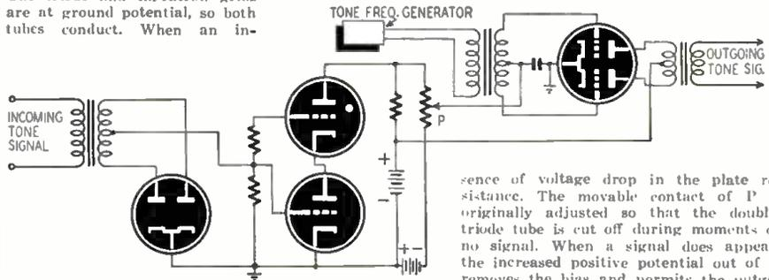
sence of voltage drop in the plate resistance. The movable contact of P is originally adjusted so that the double-triode tube is cut off during moments of no signal. When a signal does appear, the increased positive potential out of P removes the bias and permits the outgoing tone signal to be transmitted. This system allows keying of the local generator rapidly and in accordance with the incoming telegraph signal.
