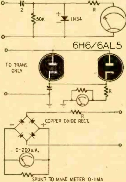
Fig. 3—Output meter rectifiers, three types. with a heavy shunt, or both. Fig. 3 shows several output meter circuits. Figs. 2 and 4 show their proper connection. (Continued on page 84)
