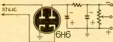
The filter constants will depend on the amount of filtering required.
