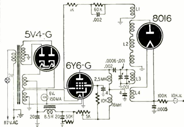
Fig. 4—An r.f. power supply. The filament also operates on r.f.
