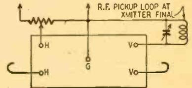
Fig. 10—Connections for modulation tests.
