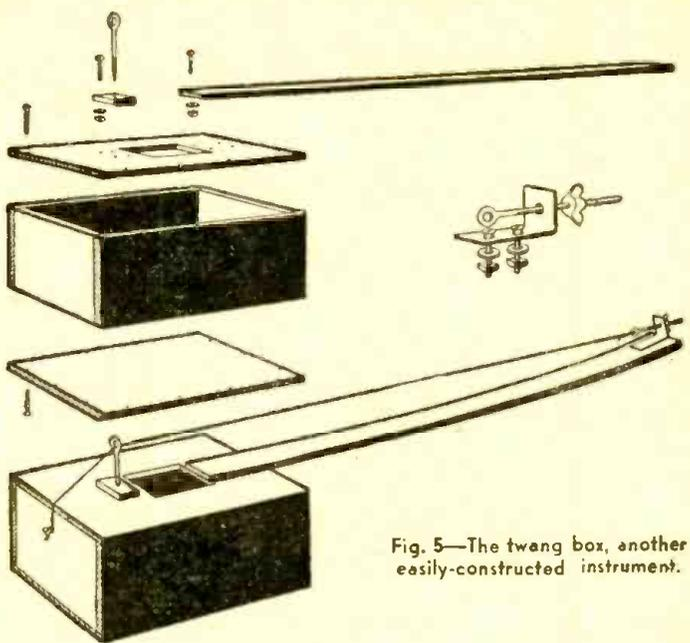
Fig. 5—The twang box, another easily-constructed instrument.
