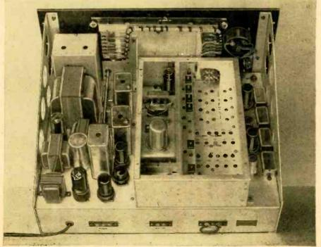
Rear view of the receiver. All tuning components are contained in the center compartment.
