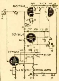
This 3-tube unit can be operated from the power supply of the average a.c. amplifier or from a separate supply.
