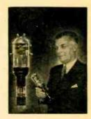
Dr. R. W. Sears of Bell Telephone Laboratories with the pulse modulation coding tube he developed.
