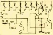
Fig. 6-Practical wide-range bridge circuit.
