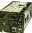
Four bands, Including broadcast (195-9.050 KC). Circuit is six-tube superheterodyne with mechanical band change or remote operated electrical band change, Remote band change and tuning controls included, making this set readily adaptable to mobile ham use. Powered from self-contained 24 V. DC dynamotor.
