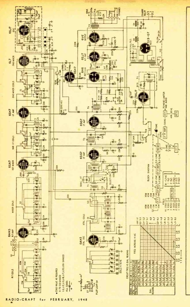
The Collins Model 75A-1, a 14-tube receiver, is designed solely for use on the amateur bands. Among a number of interesting features, it uses fixed crystal-controlled oscillators, and tunes by varying the intermediate frequencies,
