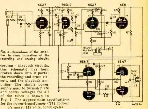
Because of the exceptionally high gain of the amplifier, it is extremely important that unusual precautions be taken to avoid excessive hum pickup. Take extreme care in the grounding circuits of the input stage. Note also that only onehalf of V2 is utilized in the playback amplifier. The other triode section of the 6SN7 (V2) is utilized in the recording amplifier, which is illustrated in Fig. 3.
