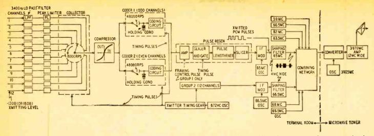
Fig. 3—The complete transmitting apparatus for one experimental circuit, indicating also how additional circuits may be accommodated.
