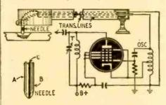
portion is very thin and therefore can vibrate much more freely than the other. As the needle follows a modulated record groove the audio vibrations cause the dielectric to be compressed and released alternately at the same audio rate. This varies the capacitance between the 2 conducting portions of the needle which are connected across an oscillator tank circuit (by transmission lines through the pickup arm.)
