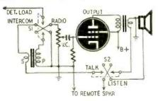
a d.p.d.t. talk-listen switch. Other leads are run to terminals for connections to the remote speaker line.
