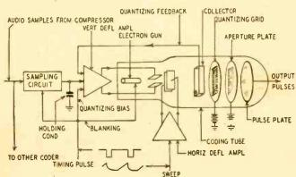
Fig. 8—The coding tube, most important feature of the system.
