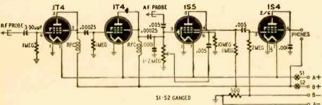
Schematic diagram. Batteries are self-contained. Note that the IS4 is connected as a triode.
