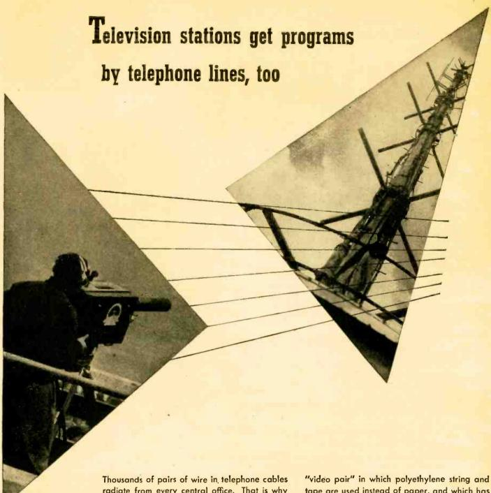
Thousands of pairs of wire in telephone cables radiate from every central office. That is why cable pairs will be handy to link cameras and transmitters wherever a television program may originate.
