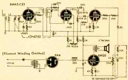
The receiver is a superregenerator with a radio-frequency stage to cut down radiation.
