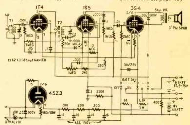
This 4-tube, 3-way portable uses 1 r.f. stage, a diode detector and 2 stages of audio.
