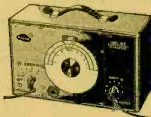
r.f., i.f., and video amplifiers. It covers a center-frequency range of 2 mc through 226 mc in 3 bands. Frequency modulation is adjustable from 40 kc to over 9 mc, and output is adjustable from zero to 1/2 volt maximum with panel controls. Synchronization of the oscilloscope, used to trace visually alignment "pictures" is at power line frequency (or selected multiple or sub-multiple), or by a 120-cycle, saw-tooth synchronizing voltage available from the generator.—RADIO-CRAFT
