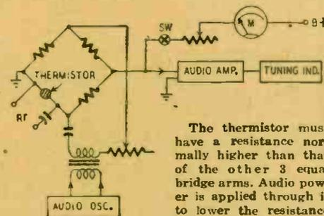
The thermistor must have a resistance normally higher than that of the other 3 equal bridge arms. Audio power is applied through it to lower the resistance and balance the bridge.
