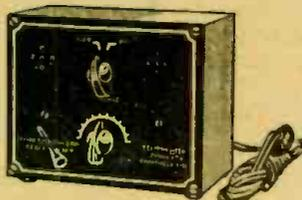
This television preamplifier boosts the strength of weak stations to a point where suitable reception is possible. It is entirely self-contained and is connected to the television set by attachment in series with the antenna. A 2-position switch on the front panel is switched on for the preamplifier or off for normal set operation.
