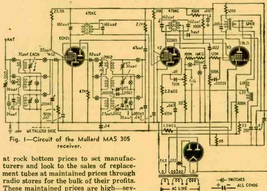
Fig. 1—Circuit of the Mullard MAS 305 receiver.
