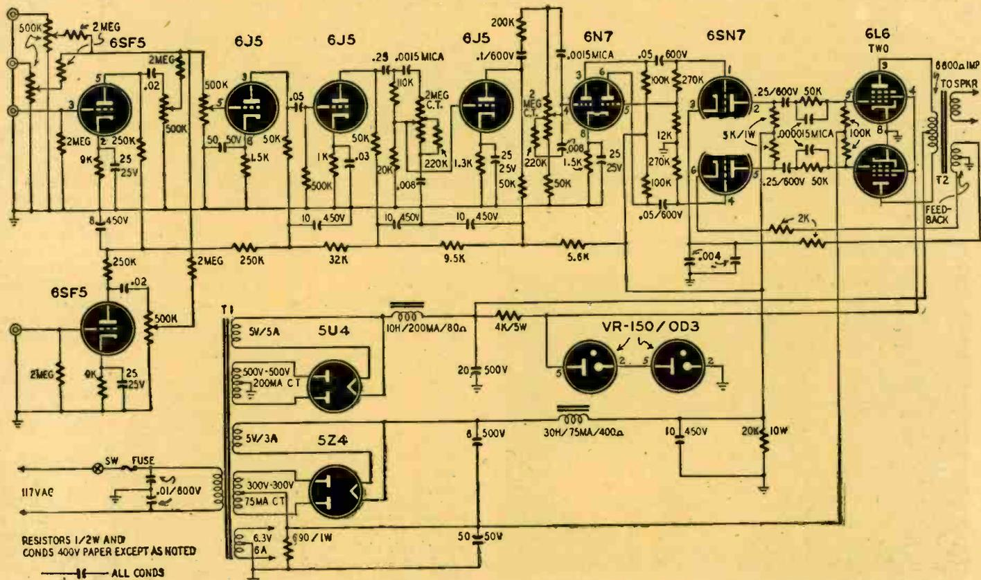
Fig. 2—The circuit of the amplifier. The bass and treble tone controls are located between the third and fifth amplifier stages.
