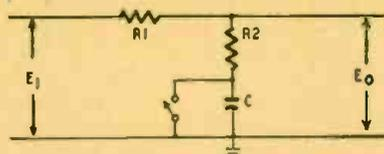
$$E_0 = E_1 \frac{R_2}{R_1 + R_2} \text{ WITH SWITCH SHORTED}$$
