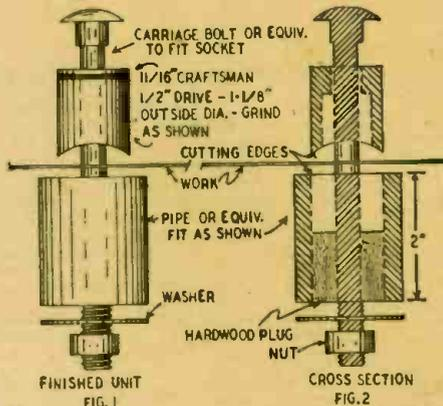
The die for the cutter is made of a piece of thick-wall pipe cut off square. It should fit snugly around cutter but not bind, if the hole is to be a clean one. Force a hardwood cylinder halfway into the pipe and drill it accurately through the center for a snug, sliding fit for the bolt.
