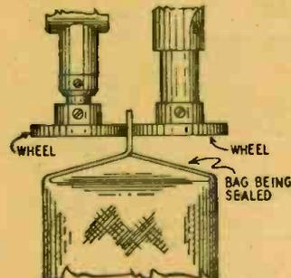
sticky. When the material is not thermoplastic, it is necessary to add a strip of film of thermoplastic substance between the sides of the bag. Again heat causes it to become sticky sealing the bag. The wheels and shafts should be of good heat-conducting material, otherwise the work (such as a bag) may overheat.
