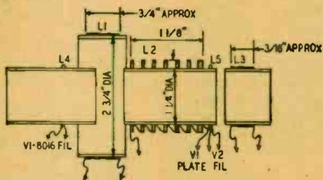
My original coil forms had 7 sections, but the coils will be flatter and neater if a larger number of sections are cut, at least 11 or 13. The forms must be cut with an odd number of sections.
