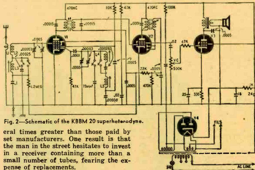
Fig. 2—Schematic of the KBBM 20 superheterodyne.
