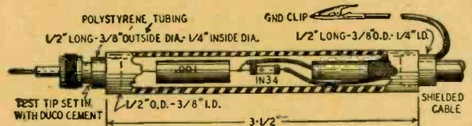
Fig. 3—This probe makes a signal tracer out of the v.t. voltmeter. The IN34 rectifies radio and audio frequency at all signal levels.
