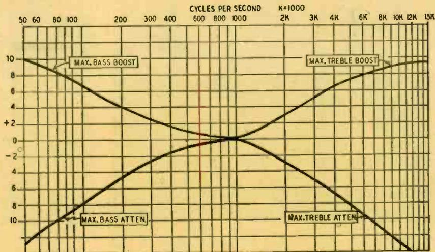
Fig. 1—Amplifier response under maximum tone control settings.
