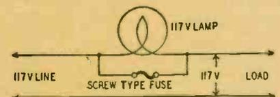
lamp should be a small one, that will not impair the action of the fuse. A  $7\frac{1}{2}$ -watt bulb is adequate.
