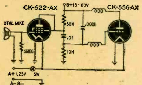
The wrist-watch radio transmitter schematic. The wrist-watch radio transmitters actually staff to build radio transmitters actually down to the size of a lipstick case (minus batteries and microphone).
