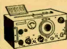
Measures frequency between 150-200 Mc. by heterodyne method. Pwr. Output of XMTTR can be measured directly. Measures DC voltages up to 500 V. Operates on 110 V, 400 cy. Complete with tubes, crystal, calibration chart. Conversion kit for 60 cy.....\$29.95
