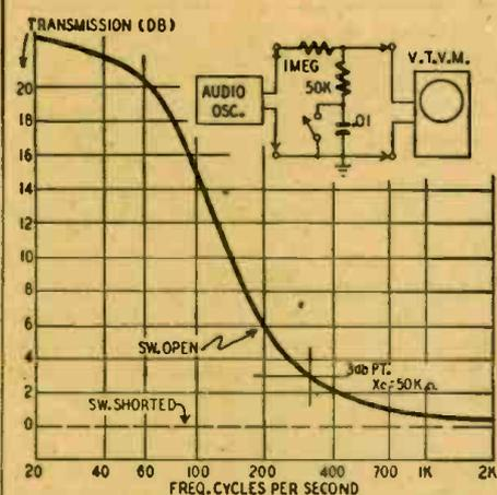
Fig. 2—Operation of the bass-boost circuit.
