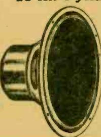
Excellent constructed high quality 15" dynamic speaker. Designed for general applications such as FM and AM receivers, fine phonographs, broadcast and recording monitoring and public address systems. 16 ohm voice coil impedance. Field 12,500 ohms. Dustproof spider and voice coil construction.
