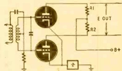
Fig. 3—Triode type; AM output from cathode.
