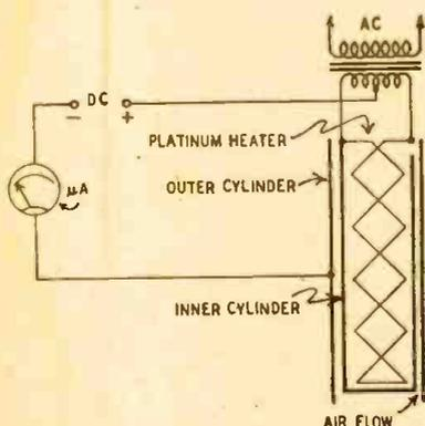
Fig. 1—Gas leaks are found with this circuit.
