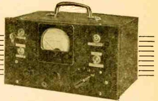
**M**ODERN radio, television, and other electronic circuits often have resistance loads of 1 megohm and higher. A meter of exceptionally high resistance is needed
