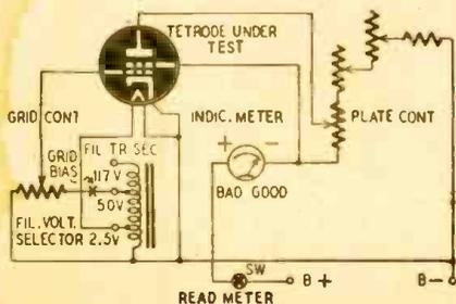
Fig. 5—Working principle of dynamic tester.
