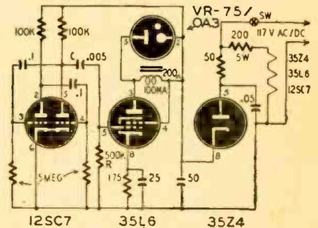
low oscillation frequency—about 1 cycle per second. The output is differentiated by the network R and C, and sharp pulses amplified by the 35L6 are developed across the output choke. A neon lamp, or in this case an OAB/VR-75 tube connected across the choke will flash briefly in step with the frequency.
