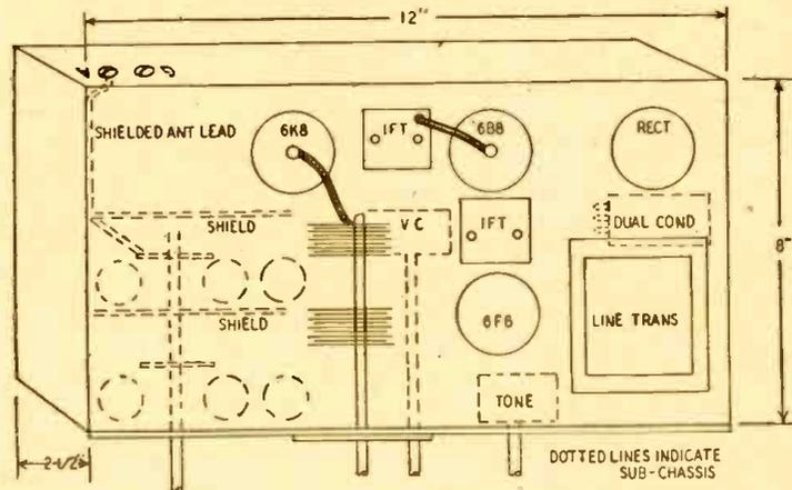
Fig. 2—Note the placement of parts. The oscillator and antenna coils are shielded.
