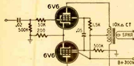
Fig. 10—One 6V6 is a paraphase inverter.
