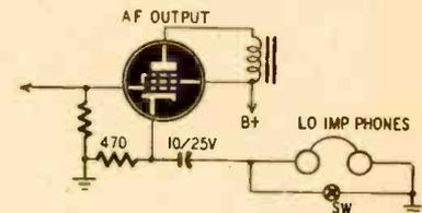
The switch across the phones cuts them out and restores normal operating conditions to the tube when the phones are not used.
