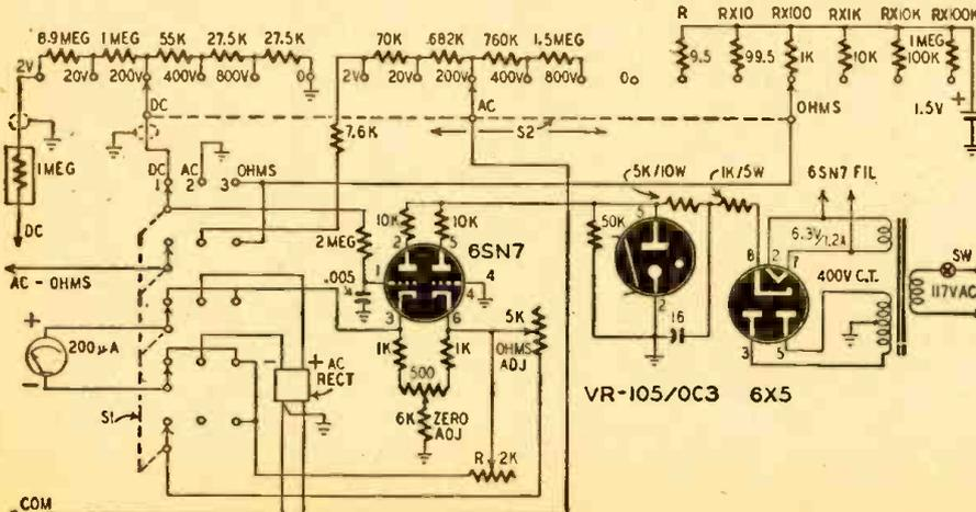
to the 2-volt d.c. scale and then touching the d.c. probe to the positive terminal of the internal dry cell. R is then adjusted till the meter reads 150 microamperes. The meter is now ready for use.
