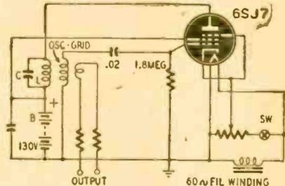
About 1 volt at 60 cycles is taken from the filament transformer and applied to the cathode to vary grid bias. Due to the non-linear tube characteristic the gain varies at 60 cycles and at various harmonics and sub-harmonics of 60 cycles. The 20-cycle sub-harmonic is especially strong because the grid circuit encourages this frequency.
