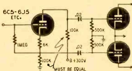
Fig. 3—Stage gain is low with this circuit.
