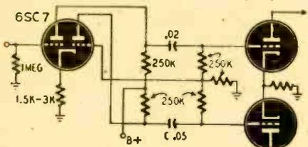
Fig. 2—The driver tube must have high gain. The signal for the inverter section depends upon the lack of circuit balance. The greater the gain of this tube, the nearer is true balance approached; therefore, a high-gain tube such as a 6SC7 is commonly used.
