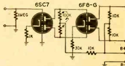
Fig. 7—A two-tube direct-coupled amplifier.
