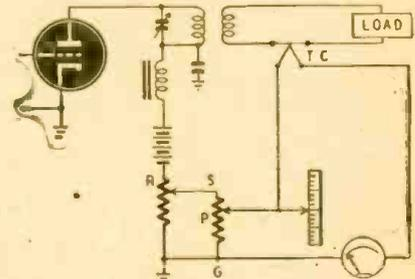
This method requires only a single d.c. galvanometer and no calculation to find efficiency. The r.f. power is measured by a thermocouple TC, which produces a voltage proportional to r.f. power. This voltage appears across PG. The d.c. voltage drop across R (and SG) is proportional to input power. The two voltages are connected to oppose each other.
