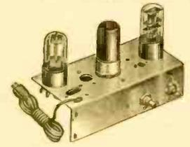
Now you can build you own hi-fidelity record player or record changer at a rock bottom minimum cost! Built-in continuously variable tone control for deep throated bass or clear toned treble output. Uses efficient 50L6, 12SQ7 audio amplifiers and 35Z5 rectifier. For 110 volt, AC-DC. Phono motor connects directly to amplifier. Complete with tubes but less output transformer. AD3-5B9584 — Less Tubes \$2.98 AD3-5B9583 — With Tubes \$4.95
