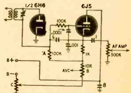
When a signal is received, diode current flows through the i.f. transformer and load to ground. The load is composed of A, B, and part of C. After filtering, only the a.f. component appears at the triode grid. This tube is used as a cathode follower. The circuits of both tubes are common, resulting in regeneration.
