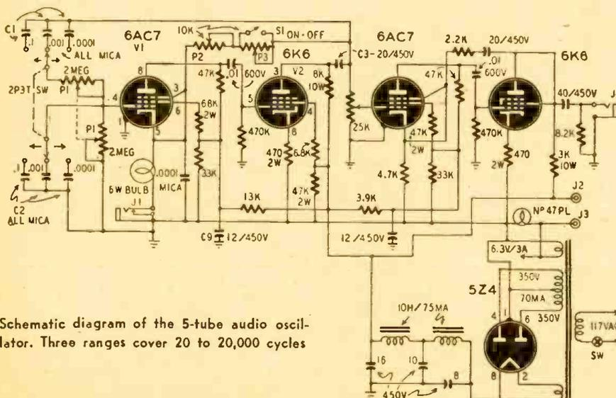
Schematic diagram of the 5-tube audio oscillator. Three ranges cover 20 to 20,000 cycles
