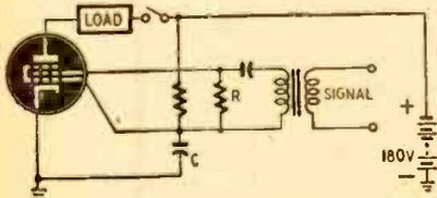
the slow charge and rapid discharge of C. Ionization is localized because a negative bias is built up on the control grid by leakage current flowing through the grid resistor. When a.c. appears on the control grid the local discharge spreads throughout the tube. A current of about 5 ma then flows from cathode to anode through the load until the switch is opened.
