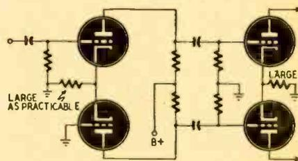
Fig. 5—The long-tailed push-pull amplifier.
