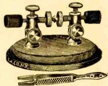
Fig. 6—The first crystal holders were offered in 1908 by the Electro Importing Company.
