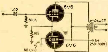
Fig. 4—The upper tube drives the lower one.
