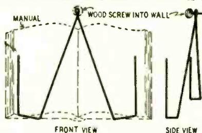
moved. A small loop is made in the wire just under the hook, and a wood screw and washer serve to fasten the loop to the wall. The remainder of the hanger is bent as shown in the drawing.
