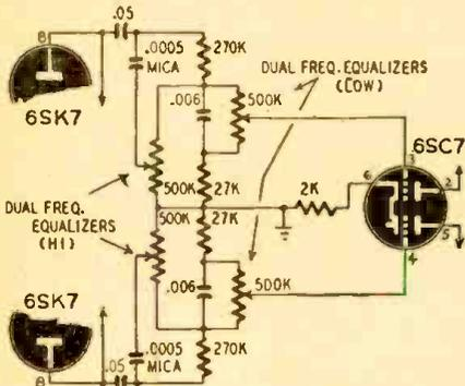
A. This circuit provides high- and low-frequency equalization. The control networks are in the grid circuits of the 6SK7. They are controlled with dual potentiometers.
