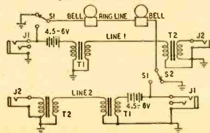
or equivalent. Switches S1 and S2 are s.p.d.t. push-button type. The normally closed contact is connected to ground. One of the two bells must be of the single-stroke type. It may be made from a standard vibrator type by connecting the line directly to the coils as shown. Do not use two vibrator-type bells.
