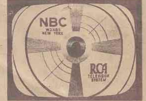
Figure 41—Vertical Linearity Control Incorrectly Set
