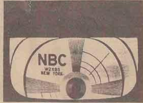
Figure 38—Vertical Centering Control Incorrectly Set
