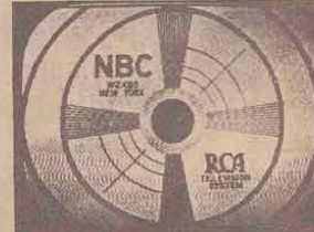
Figure 45—Excessive Diathermy Interference
