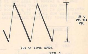
PIN 1 6SN7 VERTICAL AMP. FIGURE 21
