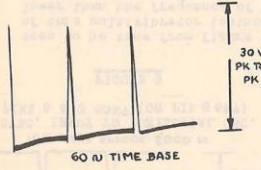
PIN 5 6SN7 VERTICAL OSC. FIGURE 16
