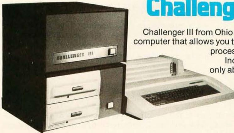
Challenger III from Ohio Scientific is the revolutionary, new triple processor computer that allows you to run programs written for the 6502A, 6800 and Z-80 processors.
